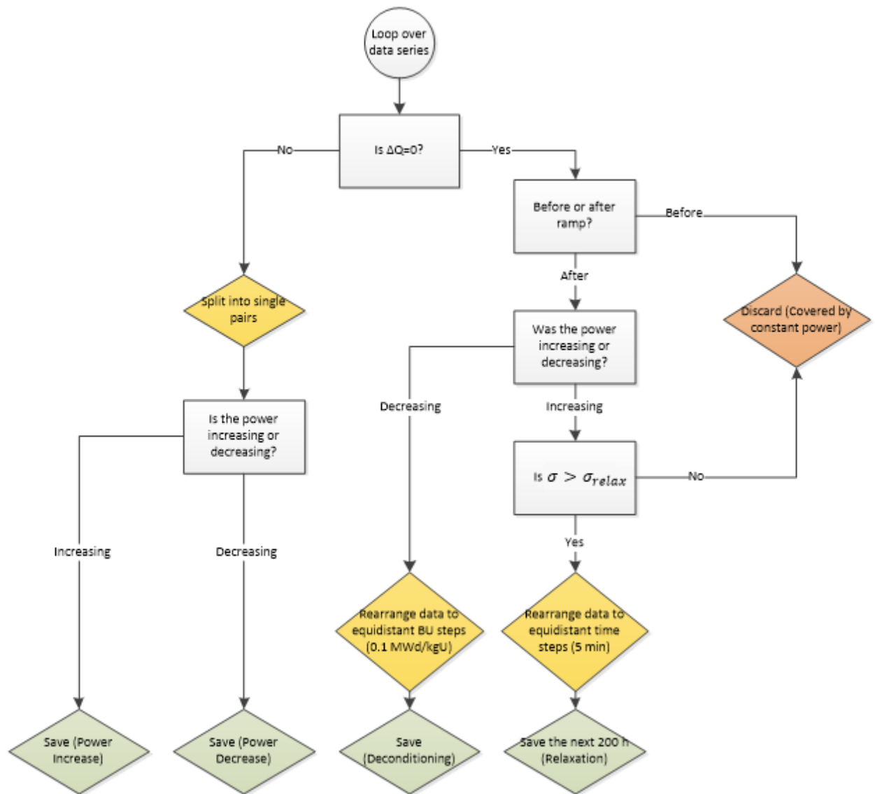
Figure 5.8- Procedure of splitting the STAV7 simulations into different cell arrays. The rectangular boxes represent decisions and the diamonds represents actions.
