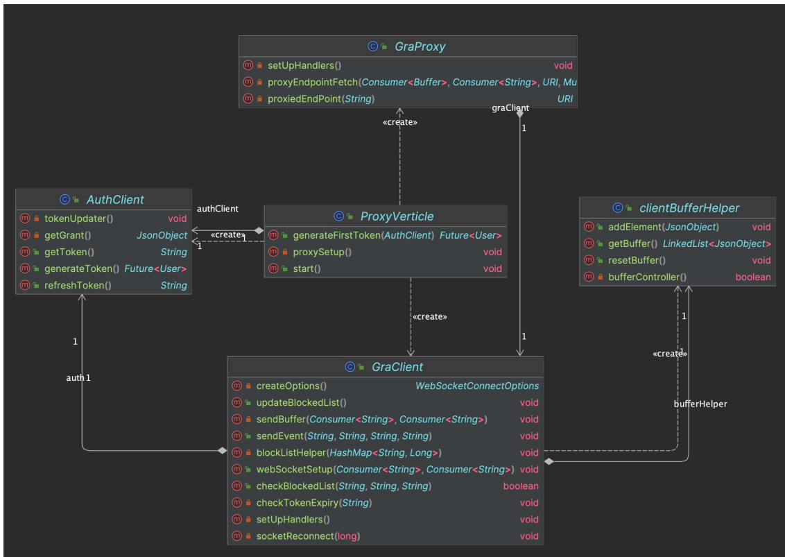
Figure 4.5: UML diagram of GraProxy
