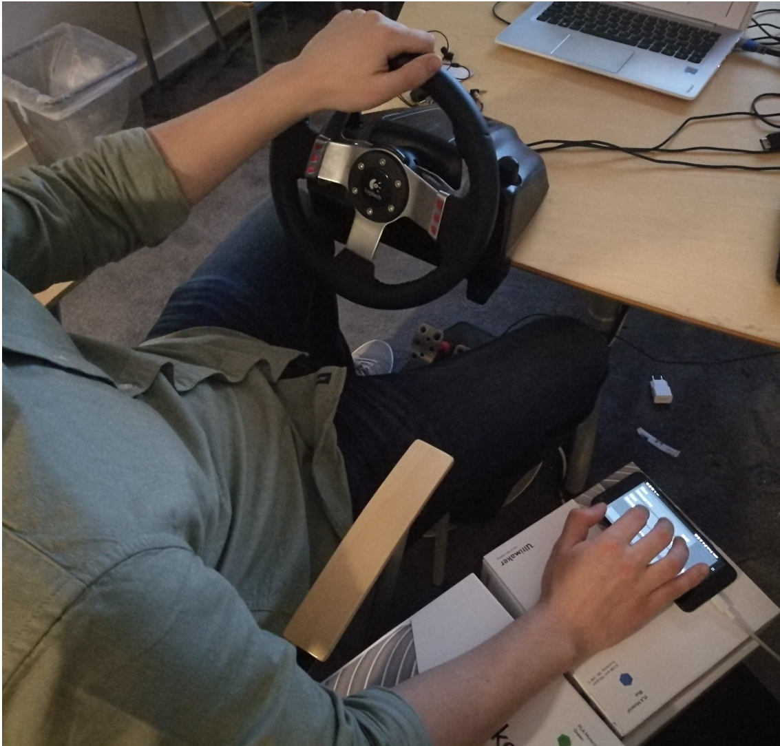
Figure 4.10: The setup for the driving simulator test using a steering wheel, pedals, and a phone as trackpad.
