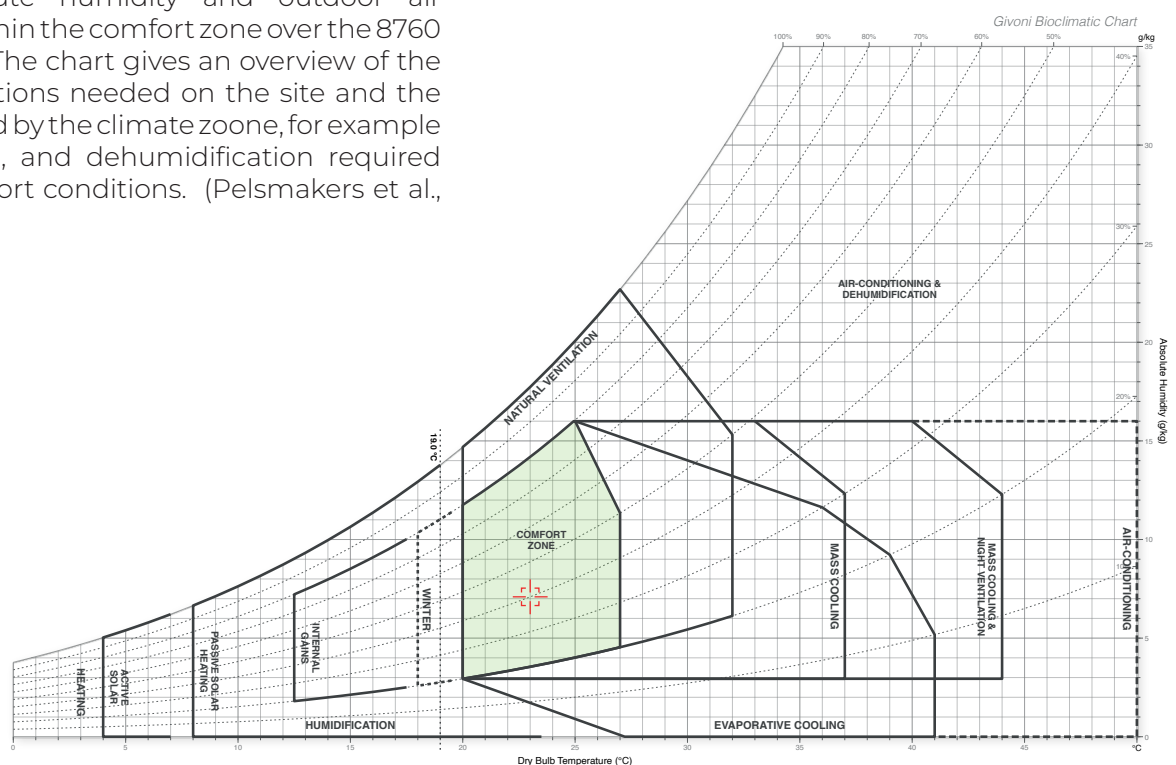
Figure 2. Psychrometric chart based on EPW data (generated using Marsh, 2018). The figure maps out how different climate areas require different solutions for indoor comfort.
