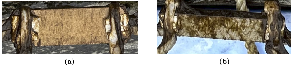
Figure 4.14: Picture taken of (a) Alloy 2 - Coating 2 and (b) Alloy 2 - Bare after 49 days of submersion.
