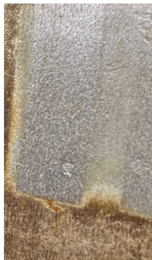
Figure 4.22: Small, visual, local corrosion attacks on Alloy 5.
