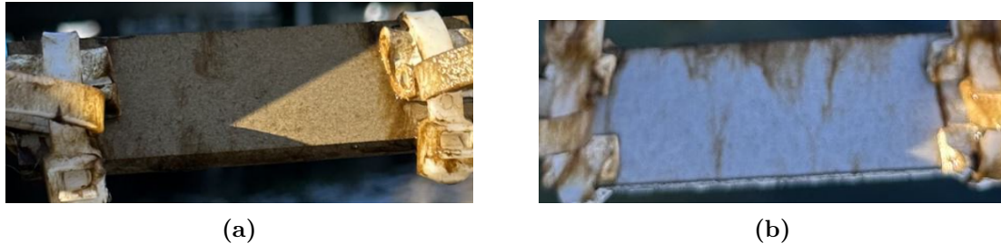
Figure 4.12: Picture taken of (a) Alloy 1 - Coating 1 and (b) Alloy 1 - Bare after 20 days of submersion.
