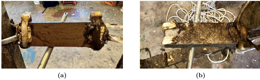
Figure 4.16: Picture taken of (a) Alloy 1 - Coating 2 and (b) Alloy 1 - Bare after 76 days of submersion.
