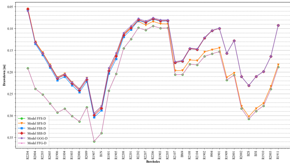
Figure 5.5: Drawdown for models with drain included after pumping in three pumping wells; B1N, BM4, B2S.
