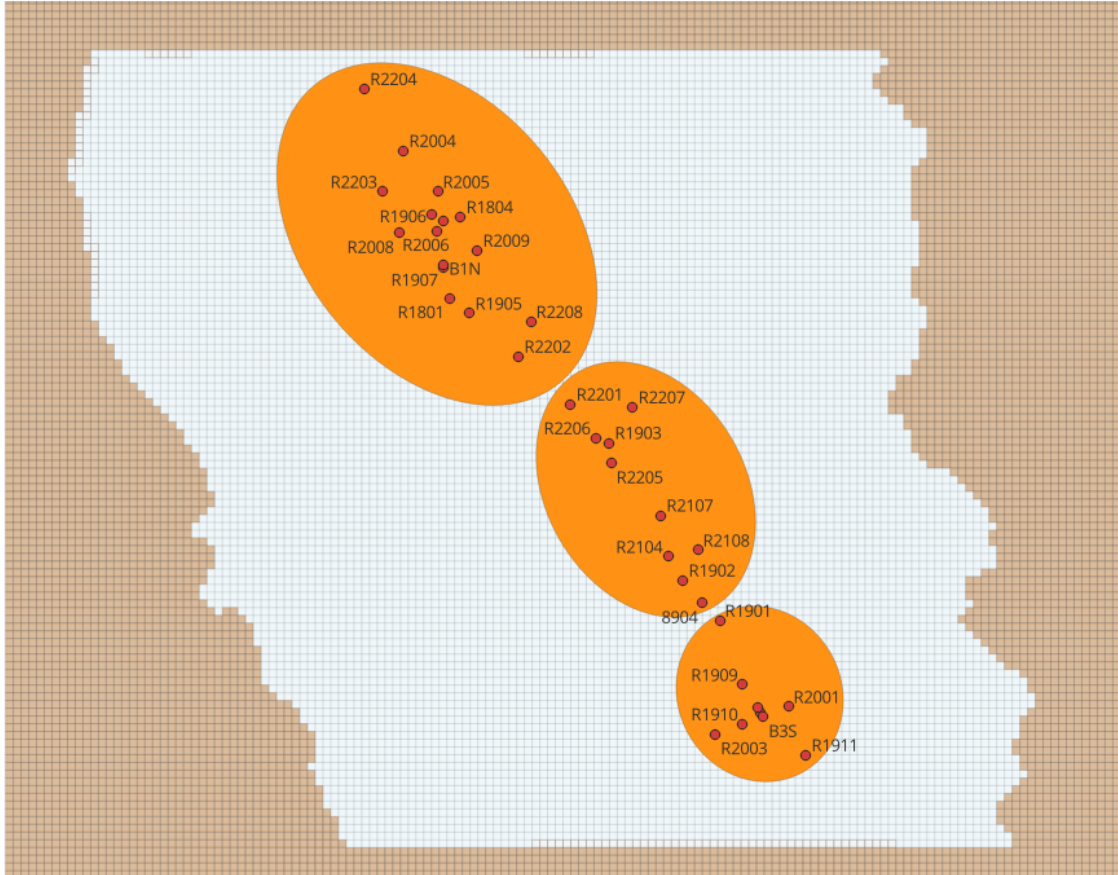
Figure 3.12: Observation wells located in the model area. All observation wells are located along the esker. The orange polygons illustrating the division of observation wells in three zones.
