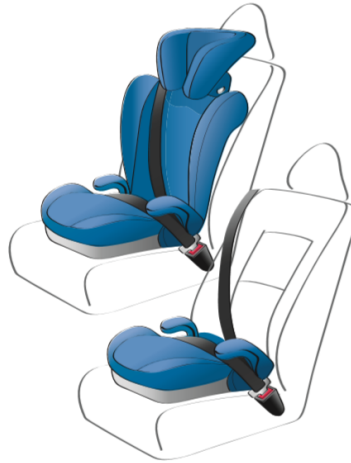
Figure 3.3: Illustration of a booster seat (top left) and a booster cushion (bottom right). [5]
