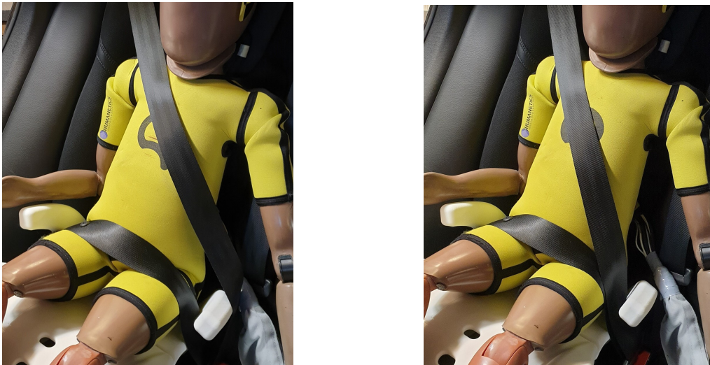
Figure 9.12: A Q6 dummy placed on a 50mm elevated SaFE prototype with belt routing over the horn (left) and under the horns (right).
