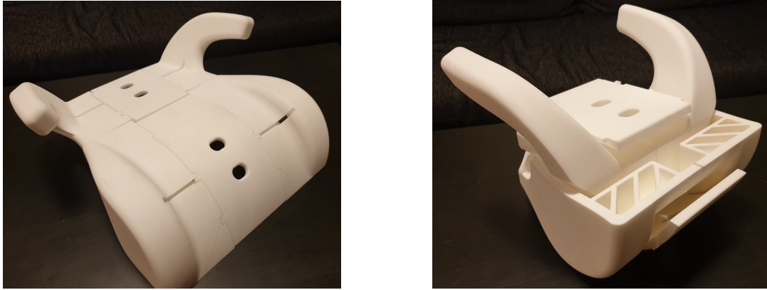
Figure 9.8: The printed prototype in its deployed state (left) and compressed state (right).
