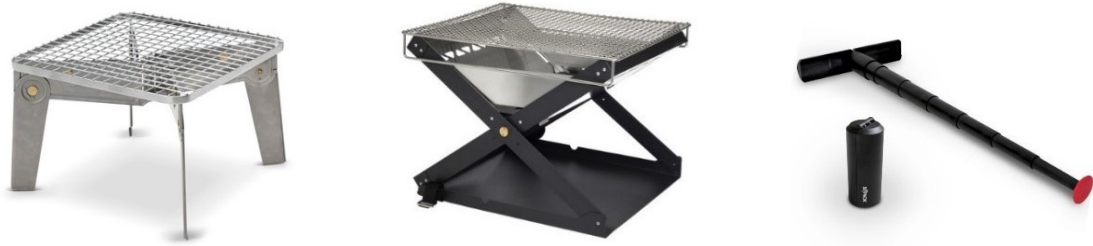
Figure 5.10: The Primus Aeryl small (left) [39] and Primus Kamoto (middle) [40] utilize sheet metal parts that fold to become small and portable. The SitPack 2.0 (right) [41] becomes smaller by retracting telescopic arms.
