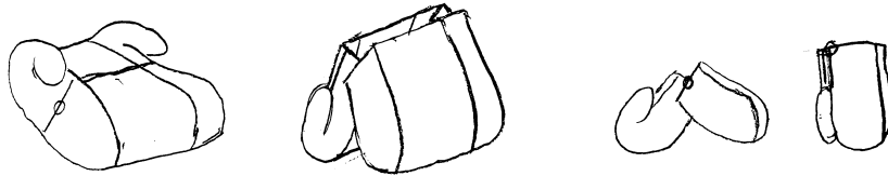
Figure 7.14: Illustration over how the Cab can be folded in half.
