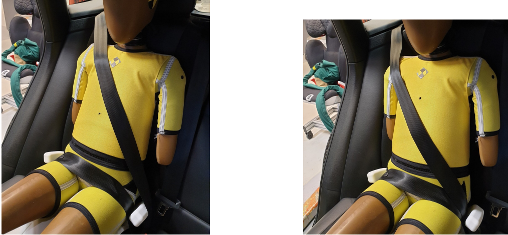
Figure 9.11: A Q10 dummy placed on a 50mm elevated SaFE prototype with belt routing over the horn (left) and under the horns (right).
