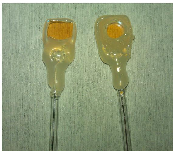
**Figure 4.3:** The electrode to the left is designed with the freehand method, and the electrode to the right is designed with a circular Teflon block to obtain a circular active surface area.
