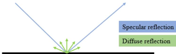
**Figure 2.1:** Considering the black line as a surface, such as a wall, the blue left hand side line represents the incoming sound wave and the blue line to the right hand side the reflected specular sound wave. It can be seen that the angle between the incident and reflected wave is 90°. The green arrows represents the diffuse reflection of the incident wave.
