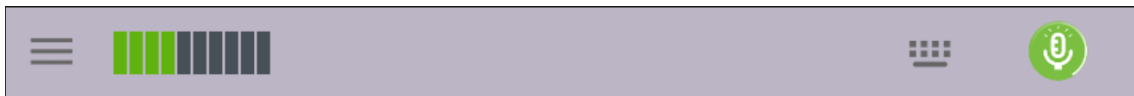
Figure 4.2: The SpeechKit control bar is added at the bottom of the speech enabled activity. The green meter to the left indicates that speech is currently registered. The color of the microphone icon to the right indicates whether the SpeechKit is listening for commands or not. Green indicates listening and red indicates not listening.
