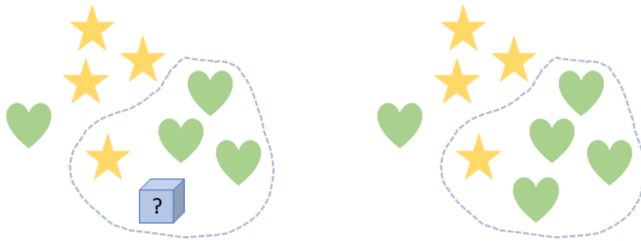
Figure 2.11: Input and output to a k-NN algorithm. To the left, the blue box is to be classified with k = 4 ; to the right, the blue box has been assigned the heart-class based on its neighbors.
