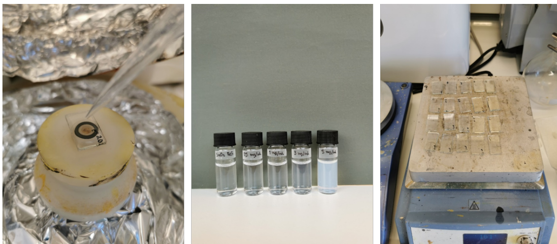
Figure 5.3: \text{SnO}_2 solution deposited onto a substrate on the spin coater (left), the \text{SnO}_2 solutions with different concentrations of the ammonium salt (middle) and substrates coated with \text{SnO}_2 solutions annealing on the hotplate (right).
