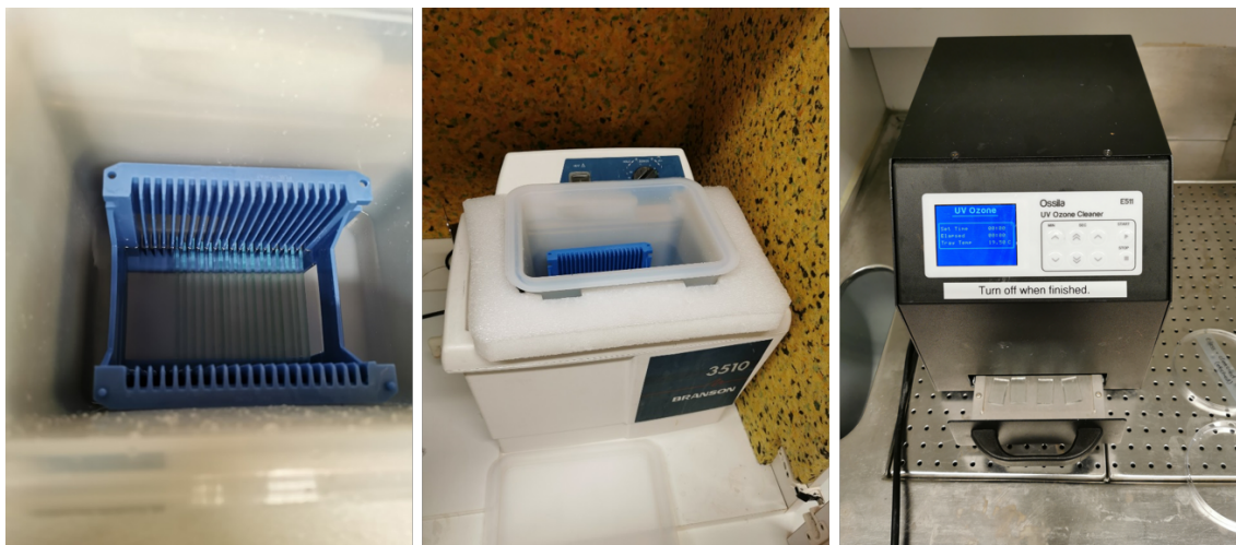
Figure 5.2: Glass substrates covered with ethanol and placed in holder (left) and put inside the sonicator (middle). The last step in the cleaning process is the UV-ozone treatment in the UV ozone cleaner (right).
