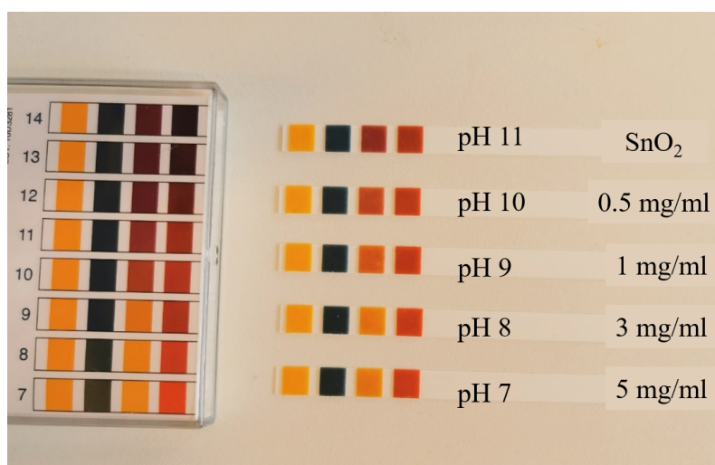
Figure 6.8: A pH measurement with pH paper of the SnO 2 solutions with ammonium salt additive.
