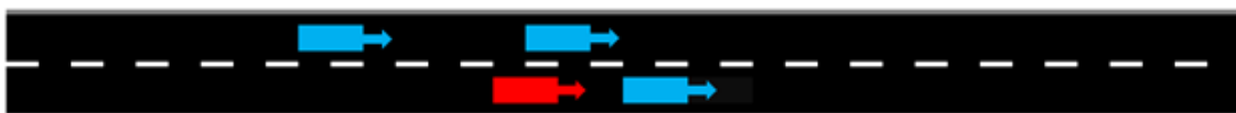
Fig. 1.3: Scenario 3, the target (blue) in front of the host (red) suddenly brakes, and two incoming targets (blue) in the adjacent lane at constant velocity.
