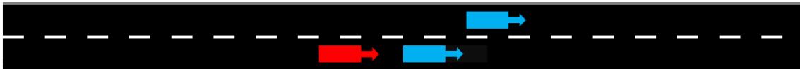
Fig. 1.5: Scenario 5, the target (blue) in front of the host (red) suddenly brakes, target (blue) in the adjacent lane.
