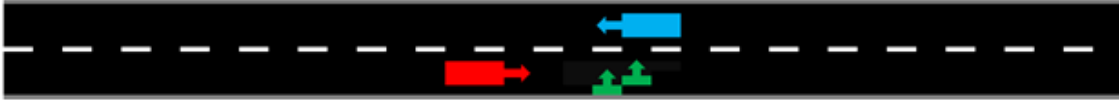
Fig. 1.4: Scenario 4, two pedestrians (green) walk out onto the road in front of the host (red), target (blue) approaches the host in the adjacent lane in the opposite direction.
