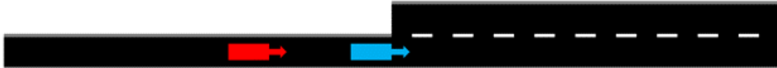
Fig. 1.1: Scenario 1, the target (blue) in front of the host (red) suddenly brakes, guardrail to the left and right, road splits up from a single lane into two lanes.
