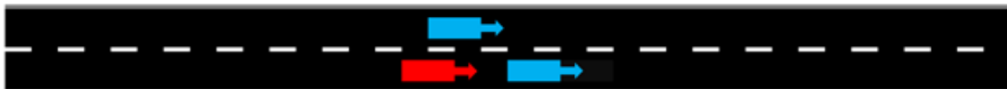
Fig. 1.2: Scenario 2, the target (blue) in front of the host (red) suddenly brakes, incoming target (blue) in the adjacent lane.
