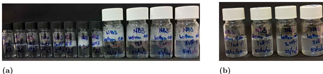
Figure 4.10: Clouding observed in PG3C10_10:1_E1: (a) at room temperature with concentrations (in ascending order from left to right) listed in Table A.x immediately after solution preparation, (b) stock solutions when kept at 4 °C for 48 hours after solution preparation (from left to right: 0.7 wt%, 1 wt%, 2 wt%, 3 wt%).
