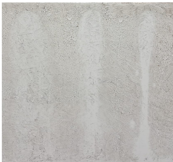
Figure 4.17: Cleaning performances of PG3C10, PG4C10 and PG6C10 (from left to right) formulations on a soiled ceramic plate.
