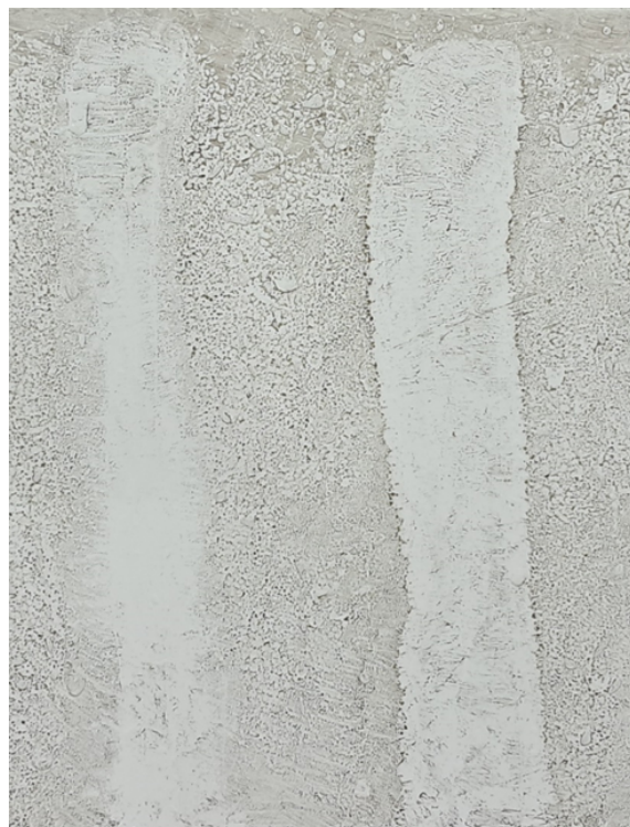
Figure 4.20: Cleaning performances of PG6C10 (left) and Berol O X 91-6 (right) formulations on a soiled ceramic plate.
