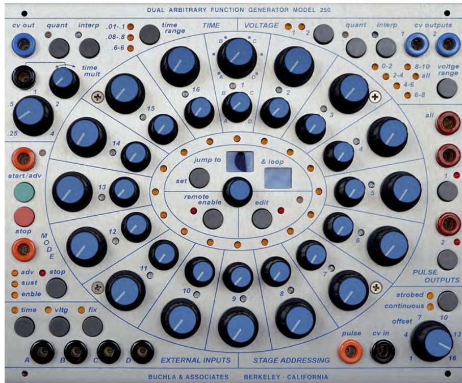
Figure 2.1: Buchla-250e - one of the earliest sequencers with a circular layout. Press photo from Buchla.
