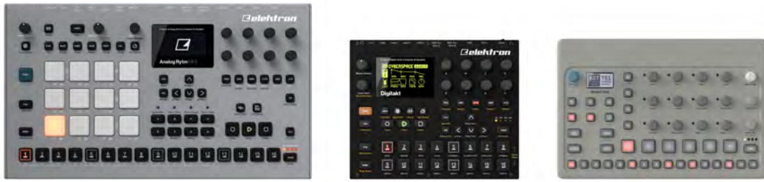
Figure 6.6: From left to right: Elektron Analog Rytm MKII, Elektron Digitakt, Elektron Model:Cycles. Press photos from Elektron. Both Rytm and Digitakt have the same type of buttons and those are considered, by some of the interviewees, better than the buttons on Roland's TR-909. Model:Cycles has rubberised buttons which IF and IA mention as undesirable.
