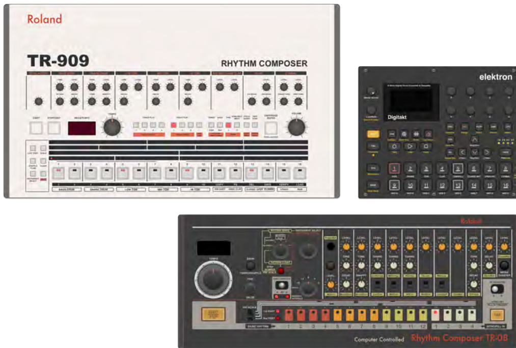
Figure 3.6: Illustration of three drum machines. From top to bottom: Roland TR-909, a synth and sample-based drum machine from 1983. Elektron’s Digitakt, a sample-based drum machine from 2017. Roland TR-08, Roland’s replica of their synth-based TR-808 from the 80s, has the same interface but in a smaller form-factor, released 2017. Notice how the step sequencer, consisting of 16 buttons in a grid or row, is present on all interfaces.
