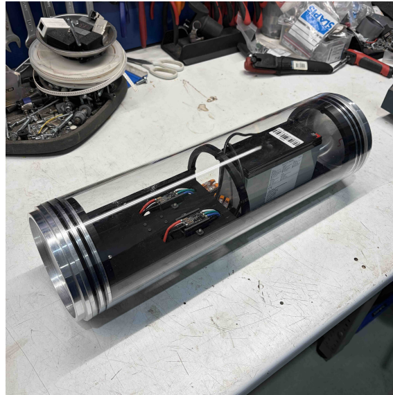
Figure 3.2: Sealed acrylic tube with internal electronics.
