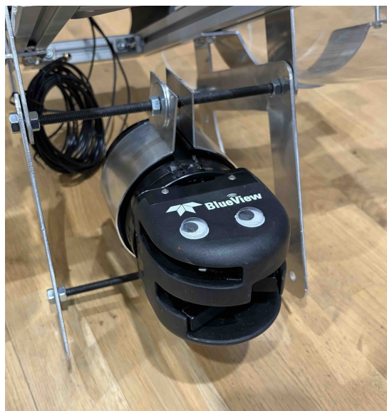
Figure 3.10: Teledyne BlueView M900 Mk2 multibeam imaging sonar.
