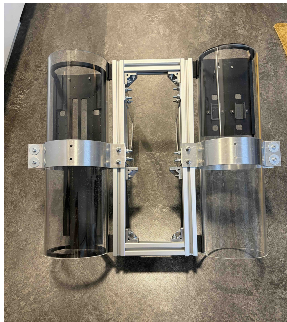
Figure 3.5: Structural aluminium frame, constructed from 3030 aluminium profiles.
