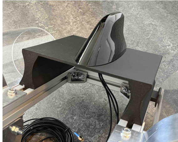
Figure 3.8: 3D-printed antenna mount.
