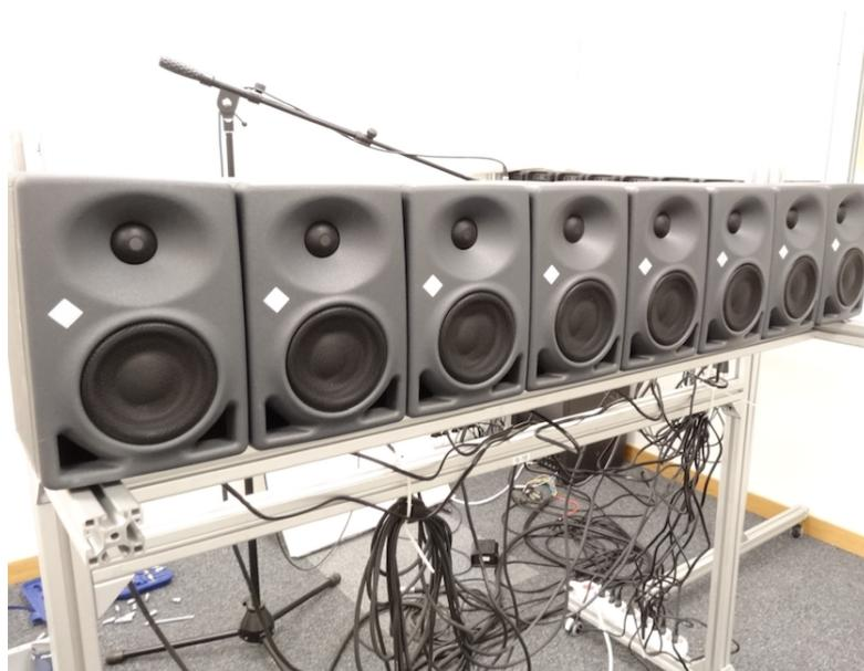
**Figure 3.1:** Example prototype using 8 *Neumann KH 80 DSP* loudspeakers with a spacing of 154 mm [19]
