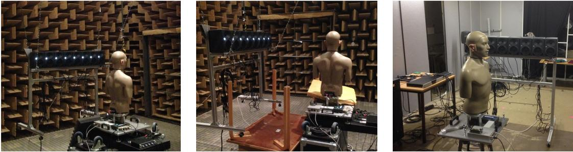
**Figure 3.10:** Photographs of HRIRs measurement setups: environment 1 (left), environment 2 (center), environment 3 (right)
