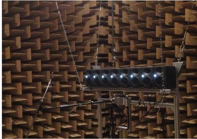
**Figure 3.8:** Photograph of the loudspeaker directivity measurement setup in the anechoic chamber
