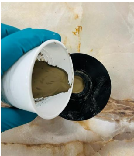
g: Fill cone with paste
