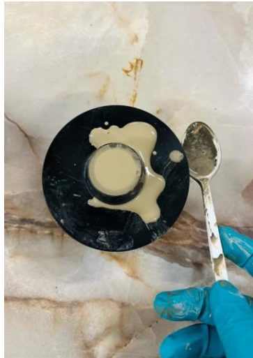
h: Tap side of cone to help settle the paste
