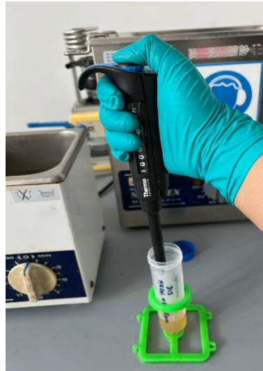
e: Pipetting 1 ml solution from top 3 mm
