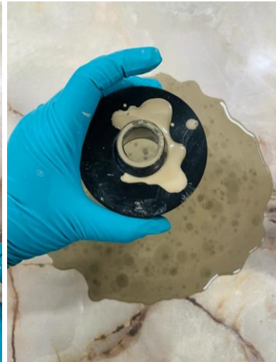
i: Vertically lift the cone and let the paste fall in a circle
