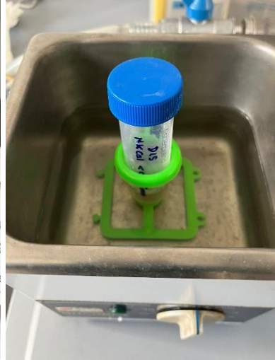
c: Sonication of suspension
