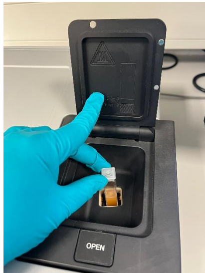
g: Putting in cuvette in DLS machine
