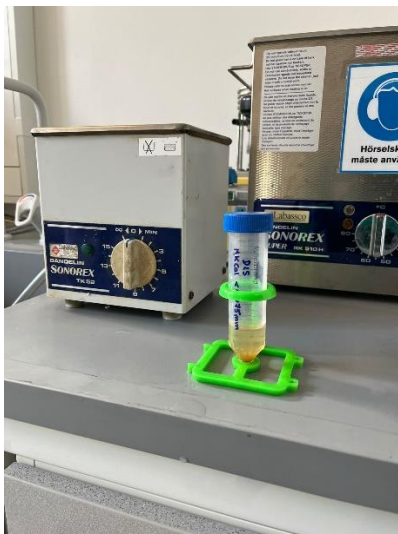
d: Settling of sonicated suspension
