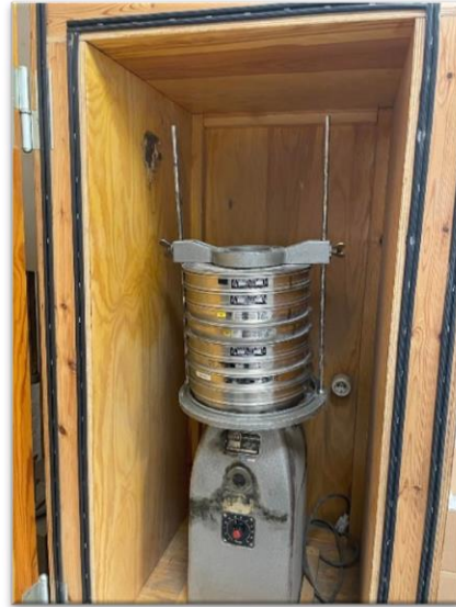
Figure 13: Sieves with clay in a shaker
