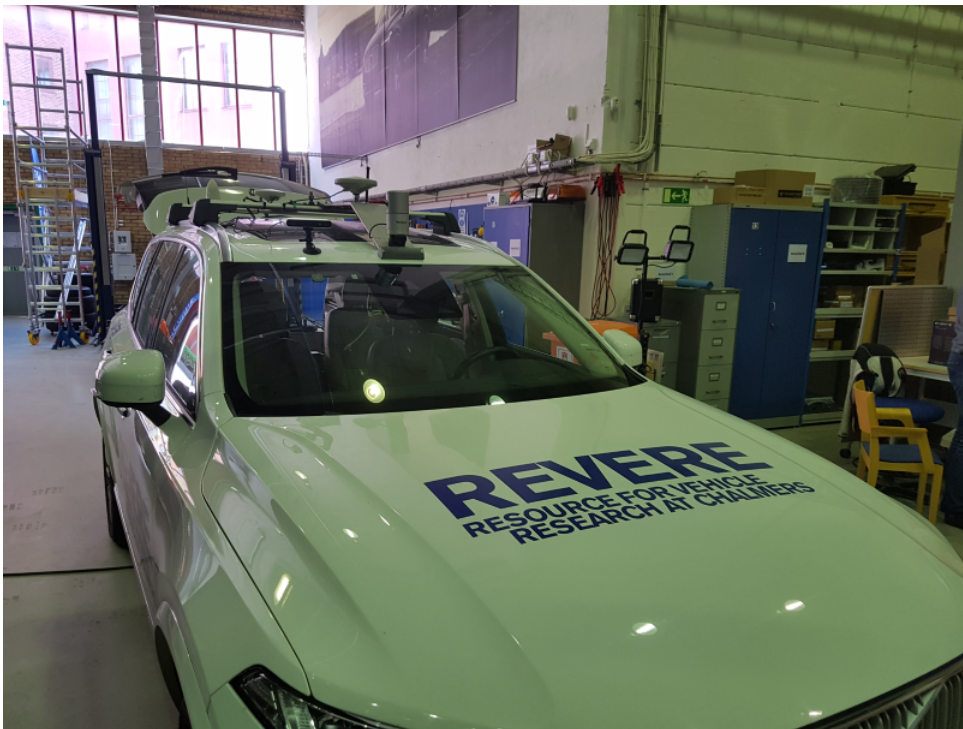
Figure A.2: Camera setup for camera position on the roof.
