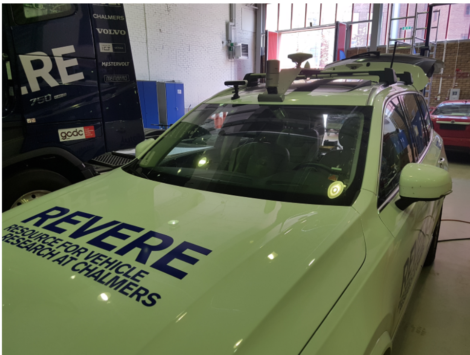
Figure A.4: Camera setup for camera position on the roof.
