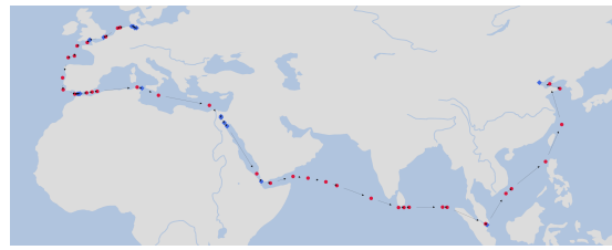
(b) Resulting A* path for the direction DEHAM \rightarrow CNTXG.
