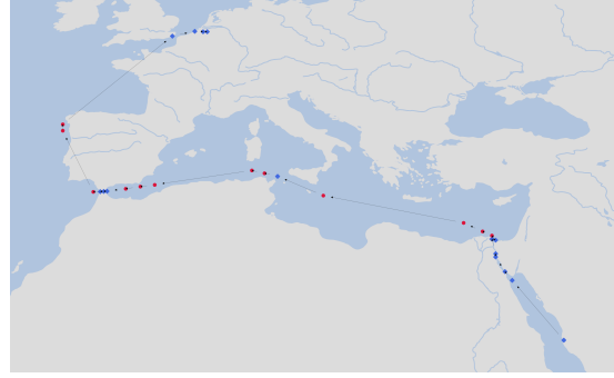
(b) Resulting A* path for the direction SAJED \rightarrow BEANR.
