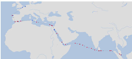
(a) Resulting A* path for the direction SGSIN \rightarrow NLRTM.
