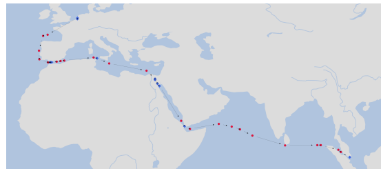
(b) Resulting A* path for the direction NLRTM \rightarrow SGSIN.
