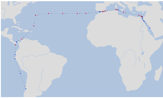
(a) Resulting A* path for the direction SAJED \rightarrow CLVAP.
