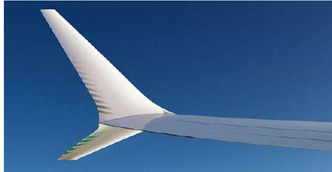
Figure 5.26: A split winglet on a Boeing 737 MAX [46].
