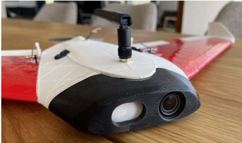
Figure 11.5: Close-up of camera installation.
