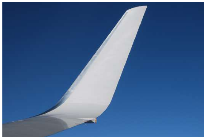
Figure 5.25: A blended winglet on a Boeing 737 [46].
