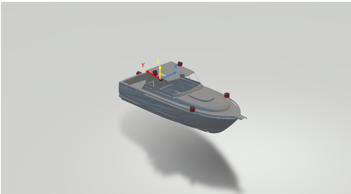
Figure B.2: Visualisation of IMU position and its coordinate system.
