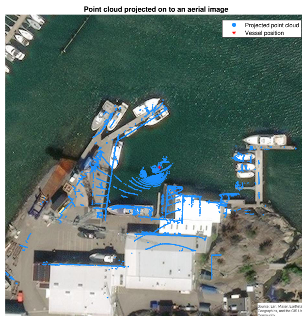
Figure 3.4: Aerial image from noisy GNSS signal with projected LiDAR point cloud as blue dots.
