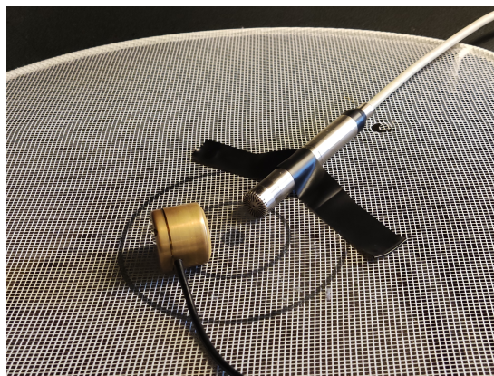
(c) microphone in anechoic chamber setup
