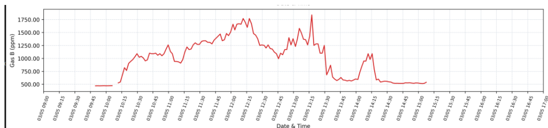
Figure A.5: CO 2 Decay Curve Measured Using Multigas Monitor
