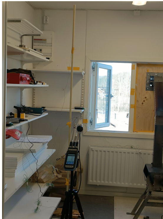
Figure 5.12: Thermocouple mounted on a vertical pole with measurement nodes N1, N2, N3, and N4, positioned in accordance with ISO 7730 guidelines.
