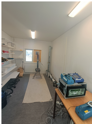
Figure 5.10: Interior view of the experimental setup showing the stove mounted onto the window board, with the chimney passing through the board. The ducting system is positioned to the right of the stove, while the extract fan is located below the duct and connected to a damper positioned in front of the fan. The measurement instruments placed on the table are also visible in the figure.
