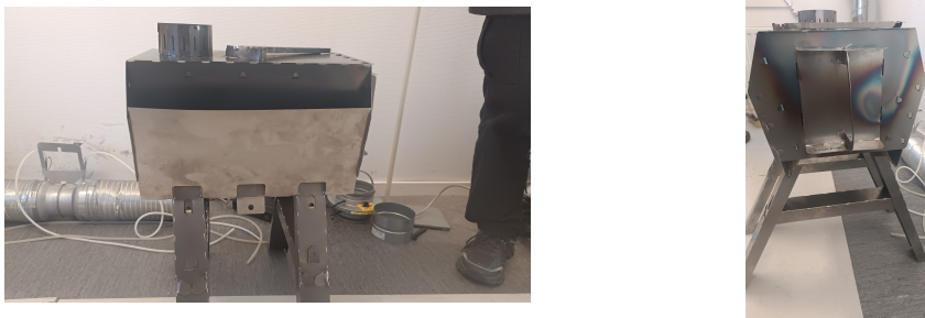
Figure 5.6: Stove assembly views: Left shows the stove side view and right shows the stove front view.
