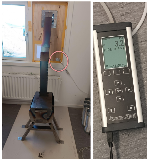
Figure 5.11: View of the tube located at the lower right corner of the window, connected to the pressure transducer for measuring the differential pressure between the indoor environment and the outside.
