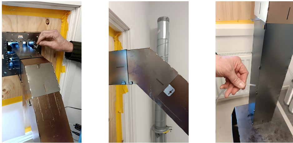
Figure 6.1: Chimney components where ultrafine particle (UFP) measurements were conducted: The left shows the horizontal chimney component, The centre shows the angled chimney component, And right shows the vertical chimney component.
