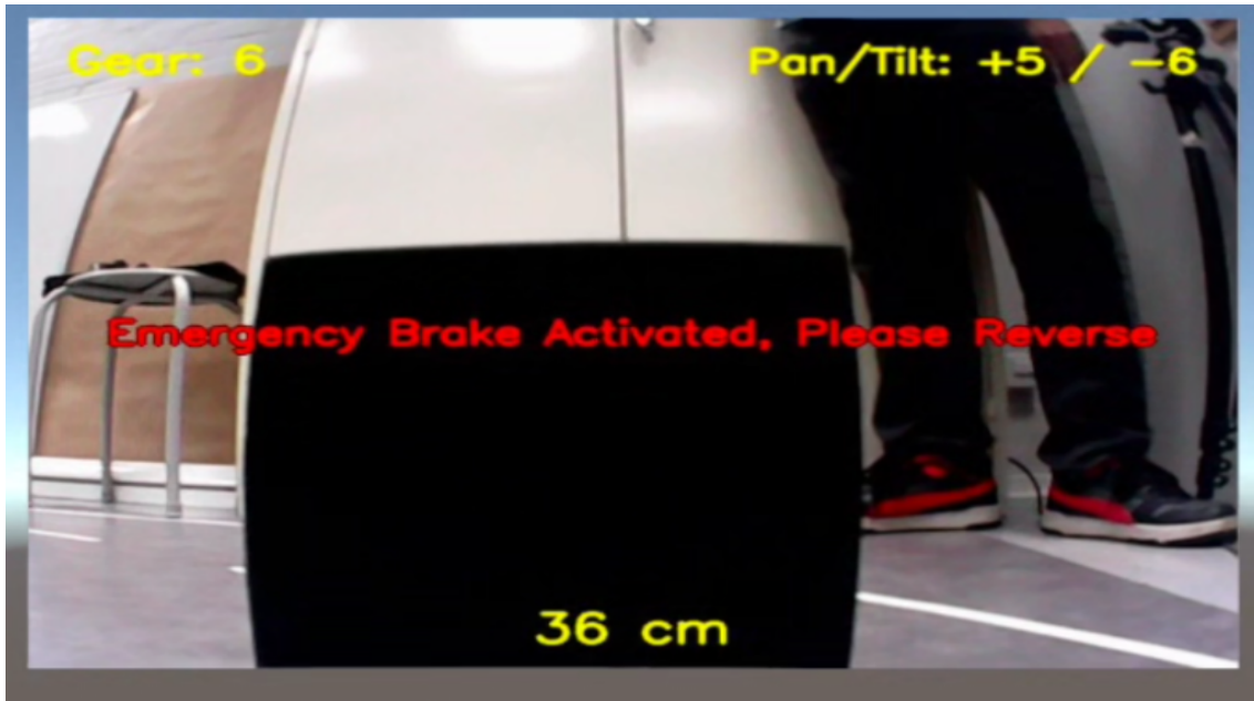
Figure 3.3: Annotated camera stream showing system state overlays: gear (top-left), camera pan/tilt (top-right), measured front distance (bottom center), and AEB warning displayed in the image center.
