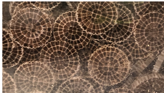
Figure 2.1: Biocarriers in operation, housing bacteria for removal of nitrate.
