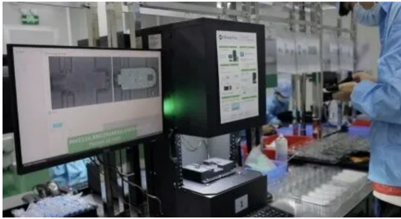
Figure 2.2: Instrumental's AI visual inspection system on an assembly line
