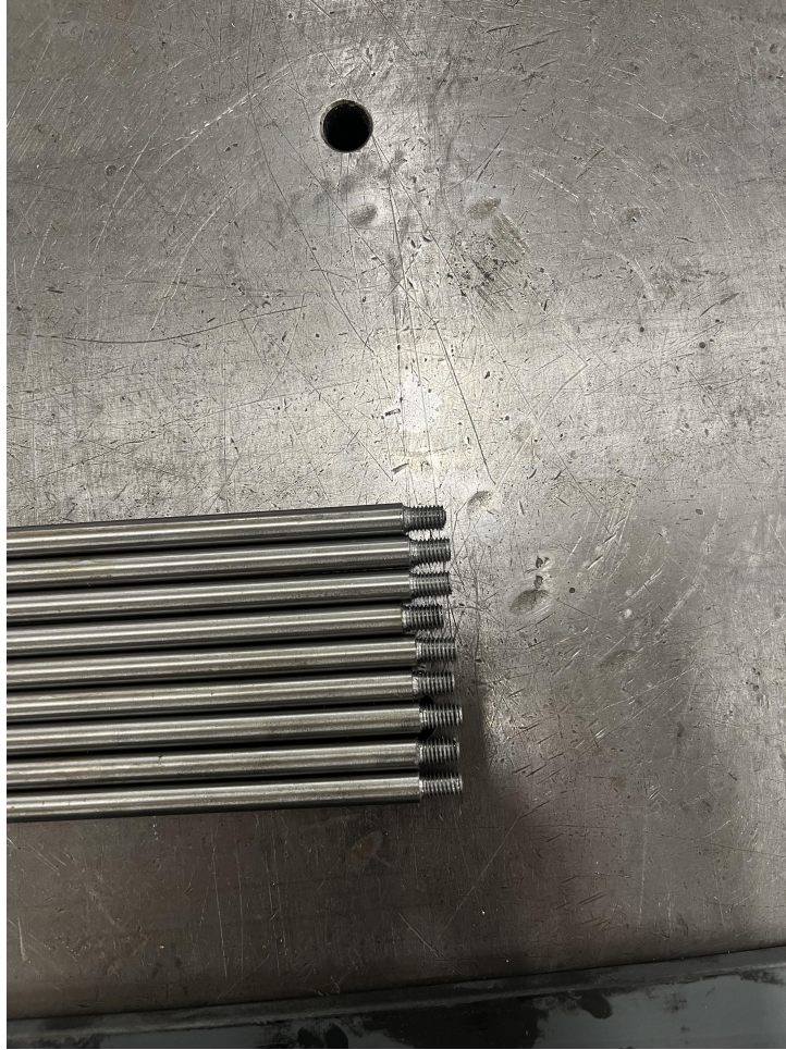
Figure 47: 8 millimeter rods lathed with M6 thread
