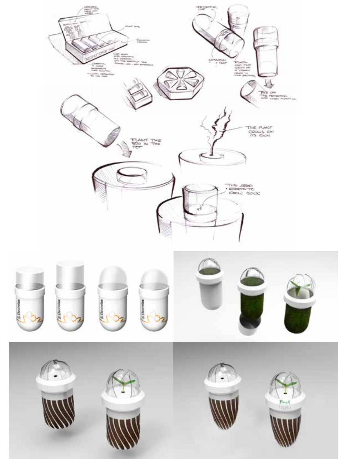
Figure 29. Hand sketches and early CAD renders of the seed pod.
