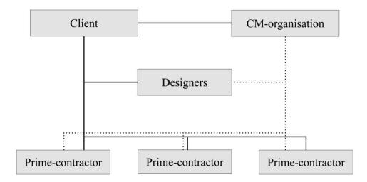
Figure 7, Organisational structure and involved actors in a CM-project in Sweden – The contract and communication relationship in a typical Construction Management approach. The dotted line indicates a communication path with no contractual relationship between the actors.
