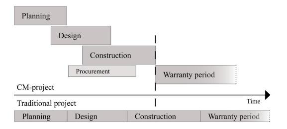
Figure 6, Project phases in a CM-project compared with a traditional construction project - In a typical CM-project the planning, design and construction phases are overlapping.
