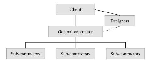
Figure 3, Organisational structure and involved actors in a design-bid-build contracts - The contract and communication relationship in a design-bid-build agreement. The dotted line indicates a communication path with no contractual relationship.
