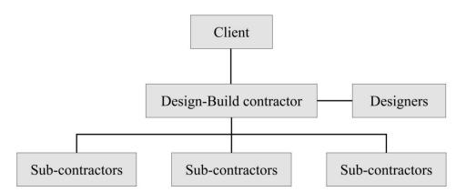
Figure 2, Organisational structure and actors involved in a design-build contract -The contract and communication relationships in a design-build agreement.
