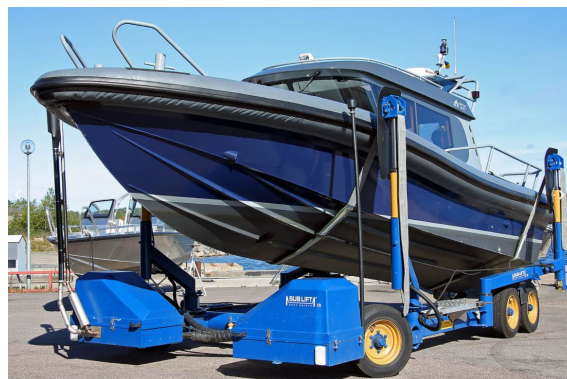
Figure 2.2: Sublift 12T model lifting a boat.
