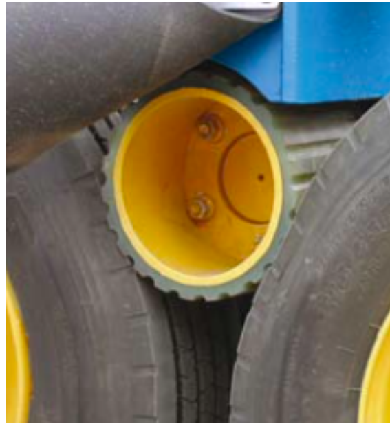
Figure 2.3: Robson drive roll mounted in between the rear wheel pair.
