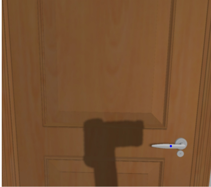
Figure 13: The closest point on a detected handle object represented by a blue dot
