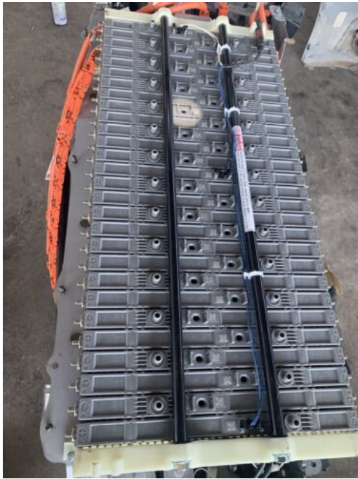
(a) New Toyota Prius battery module [19]
