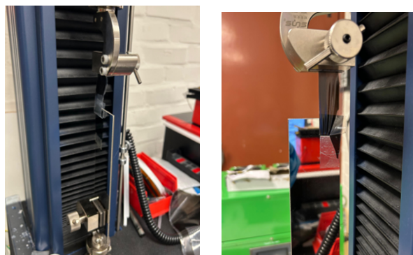
Figure 4.10: Adhesion test setup for PA film. The experimental configuration showing (left) film alignment in UTM grips and (right) peeling during load application.
