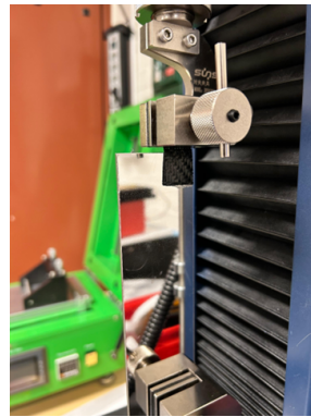
Figure 4.12: UTM test setup for carbon fiber adhesion testing
