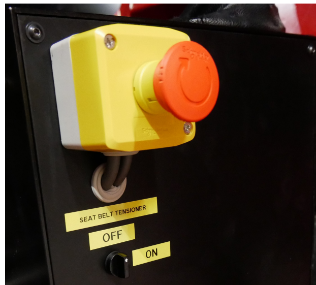
Figure 3.7: Side panel with power switch and emergency stop
