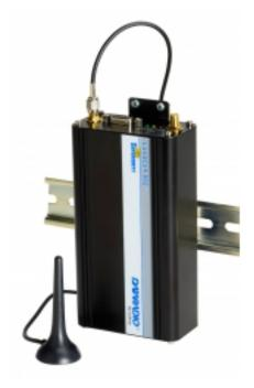
Figure 5.3: CalAmp LandCell-882 GPRS modem
