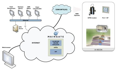
Figure 4.3: mVio Internet SCADA, architecture
