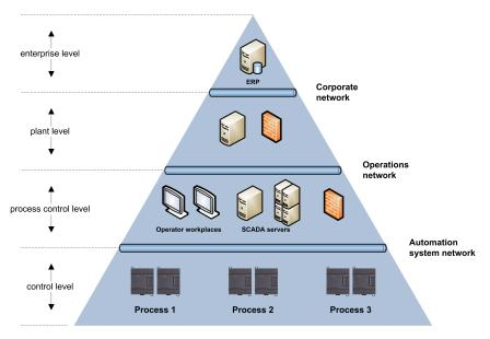
Figure 3.3: Industrial control system architecture
