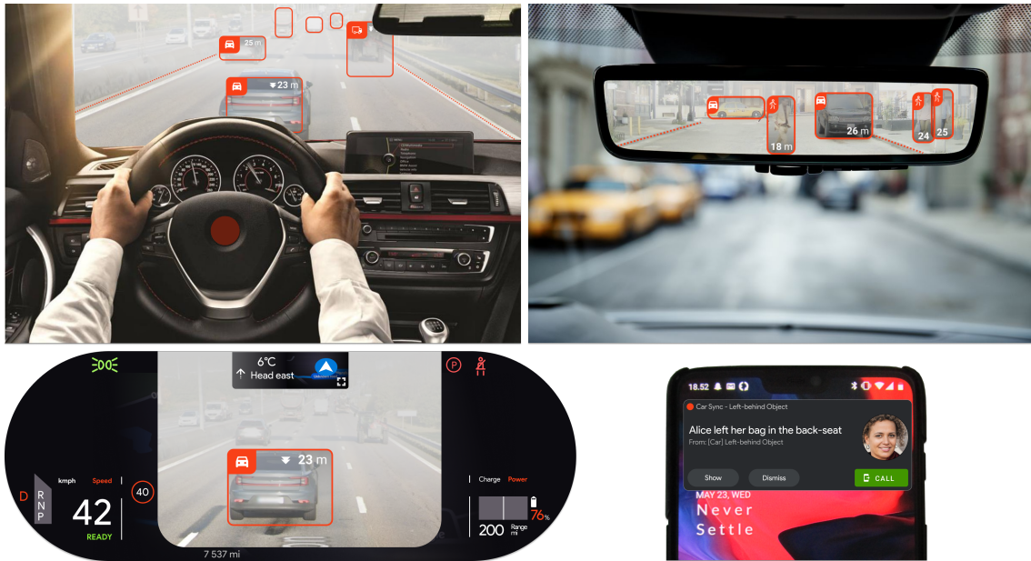
Figure 8.3: Additional visual spaces where the artefacts could be realized in the future. Clockwise from left, ADASight as a Heads-up Display, ADASight on the rear-view mirror, LeBO phone notification and ADASight on the digital instrument cluster.
