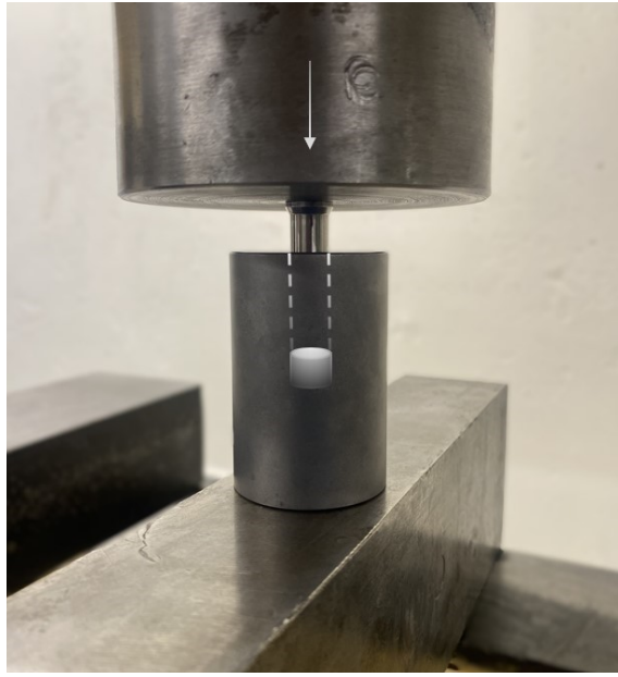
Figure 3.3: Pressing setup. As the hydraulic press is lowered, the powder of the composite is pressed into a coin-shaped pellet. The added pressure was equal to around 8 ton and were applied for 30-60 s.
