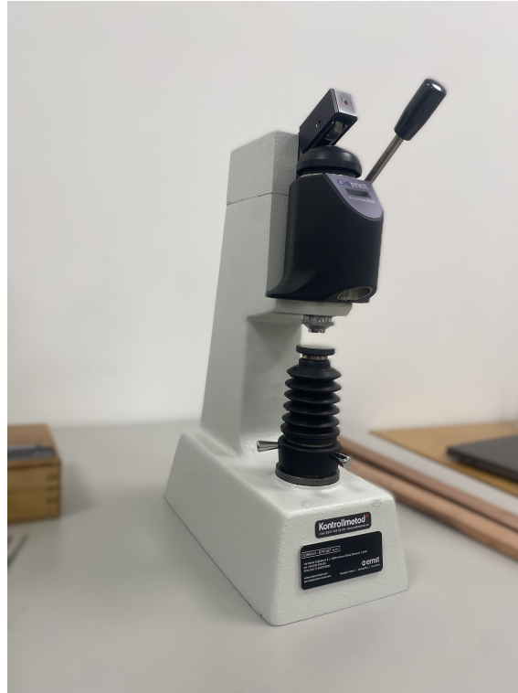
Figure 3.8: The hardness tester measured the hardness of the samples using a ball indenter in the HRB Rockwell scale.
