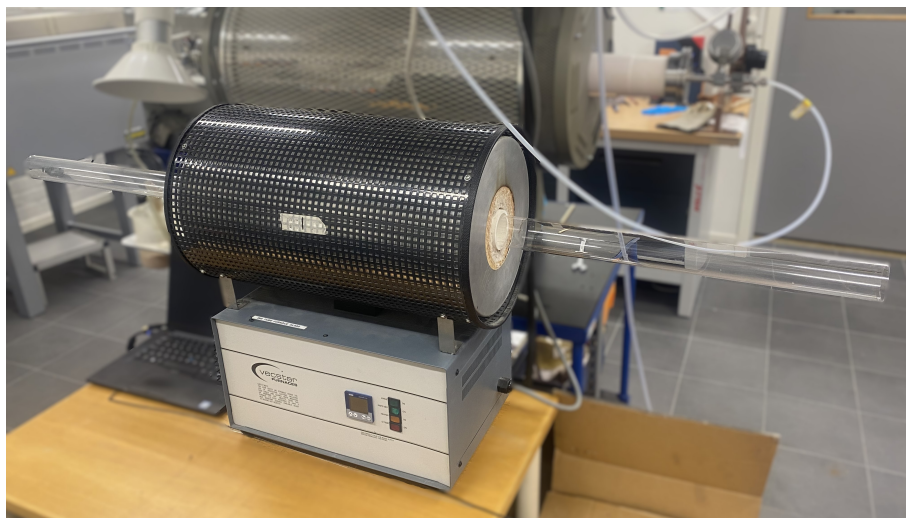
Figure 3.4: The quartz tube furnace used for the sintering process of the Al/MXene composites in argon atmosphere.
