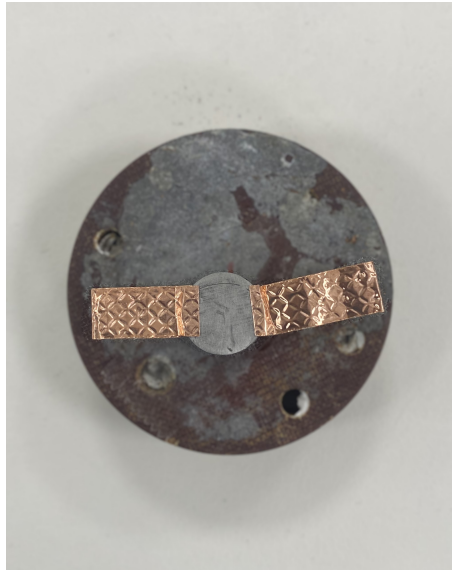
Figure 3.7: Close up over the copper wings connected to the sample. This is a way to facilitate electrical contact during electrical resistance measurements.
