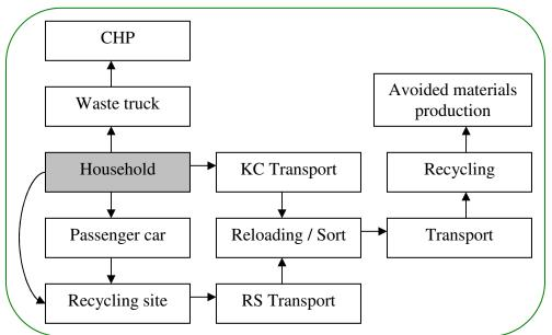
Figure 3.1 Simplified flowchart of the Bring collection system.
