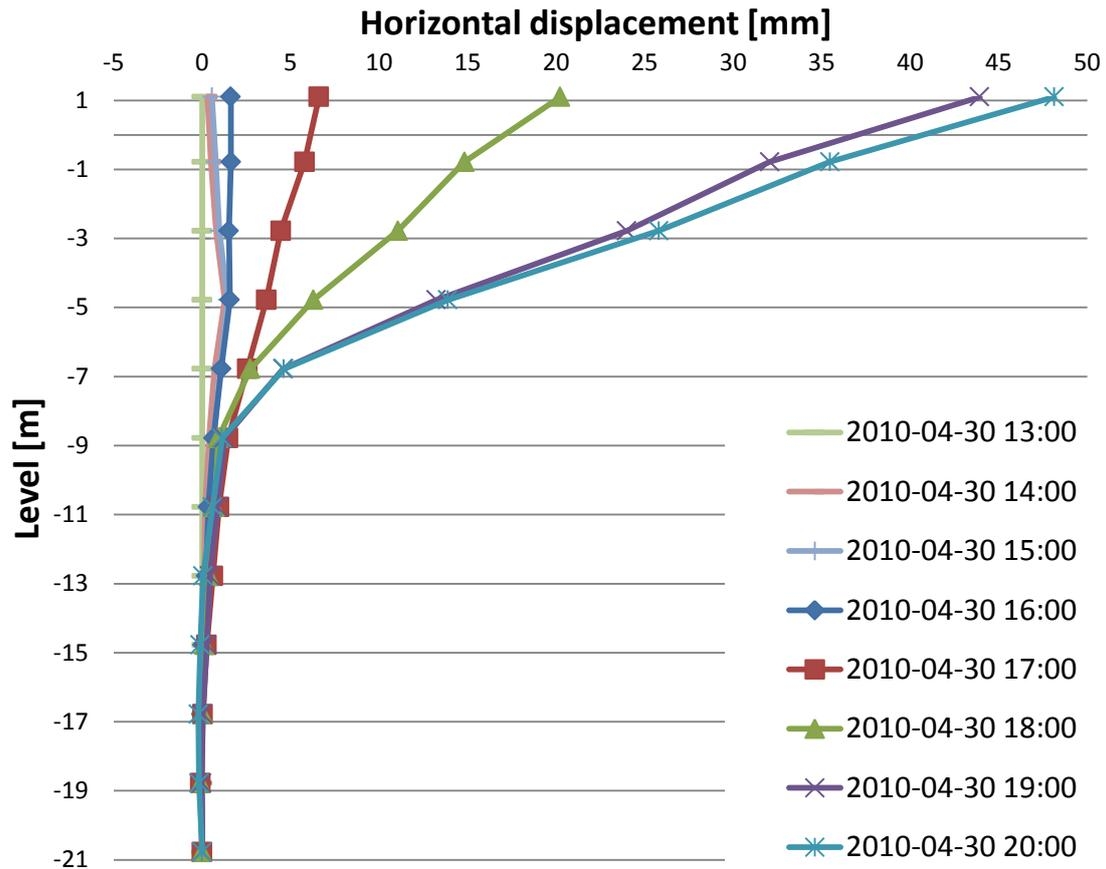
Figure 7.3 Horizontal displacements in section 465/300 during the installation of LC-columns under the would-be service road.
