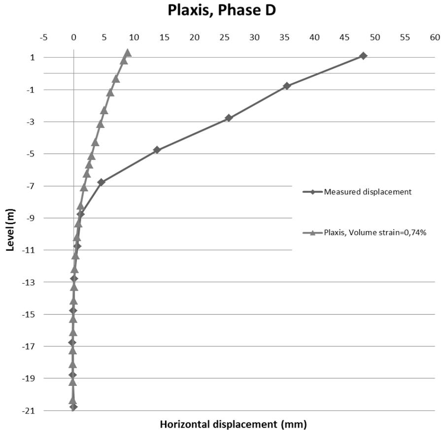
Figure 9.3 The horizontal displacements calculated in PLAXIS compared to the measured displacement in section 465/300.
