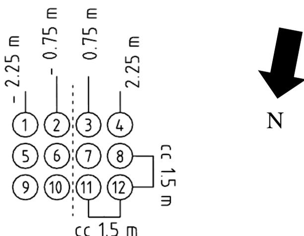
Figure 6.1 Installation order and installation pattern for LC-columns under the service road.
