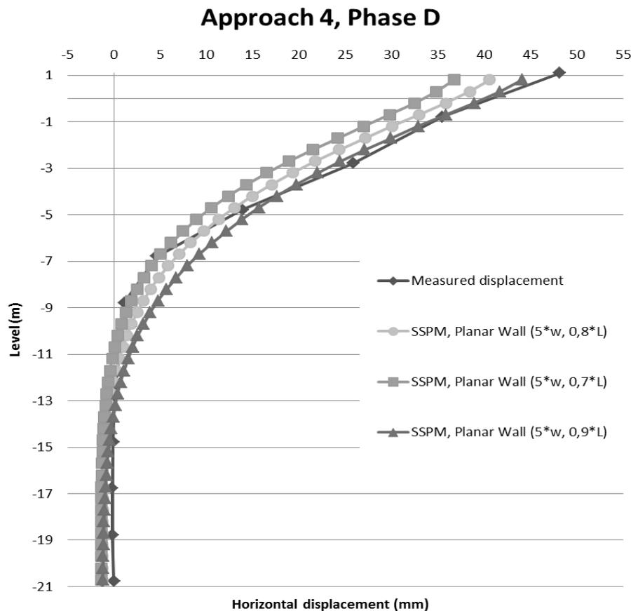
Figure 8.8 Horizontal displacements in Phase D, Approach 4.
