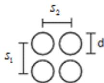
Figure 8.5 Geometry and notations for calculation of the coverage ratio of LC-columns in the column area.
