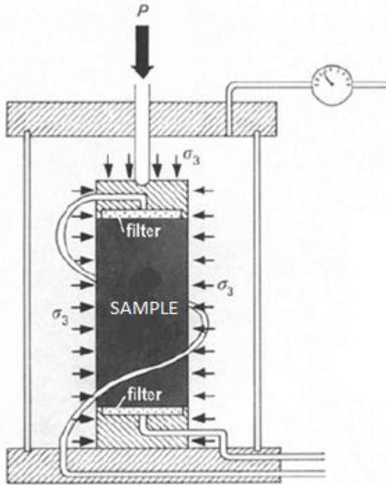
Figure 3.3 Principal sketch of a triaxial test (Larsson, 2008, modified).
