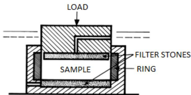
Figure 3.1 Principal sketch of a CRS test (Larsson, 2008, modified).
