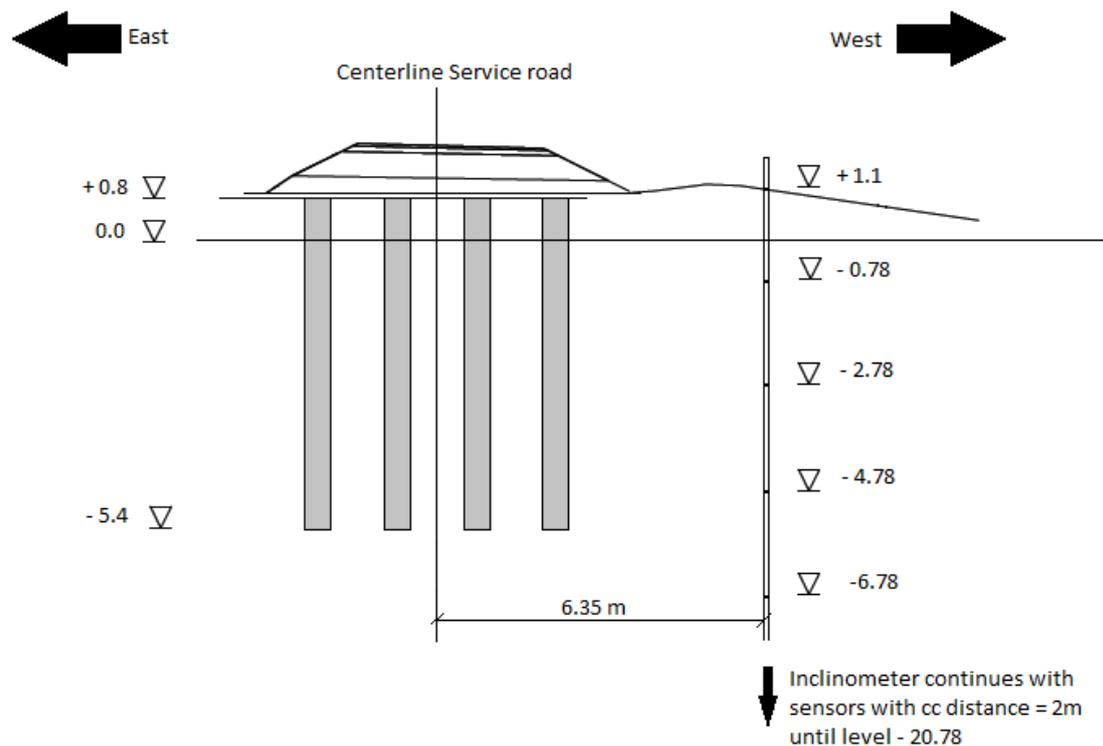
Figure 7.1 Location of the automatic inclinometer and the levels of the sensors.
