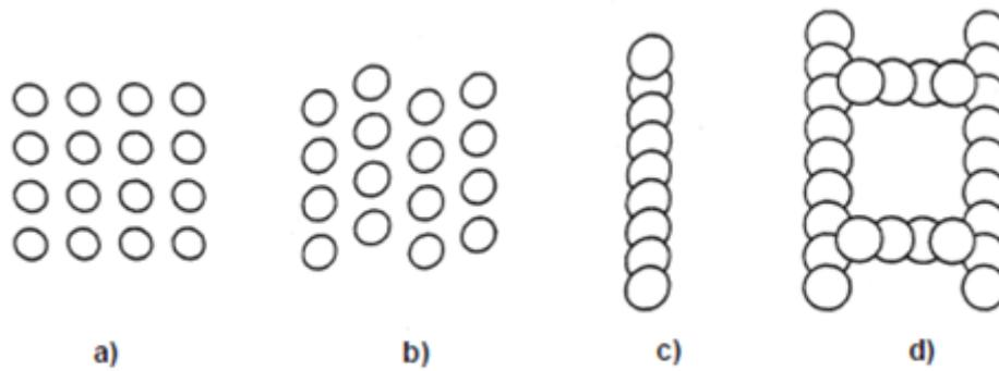
Figure 2.3 Different types of installation patterns a) Rectangular pattern b) Triangular pattern c) Panel d) Lattice (Larsson, 2006).
