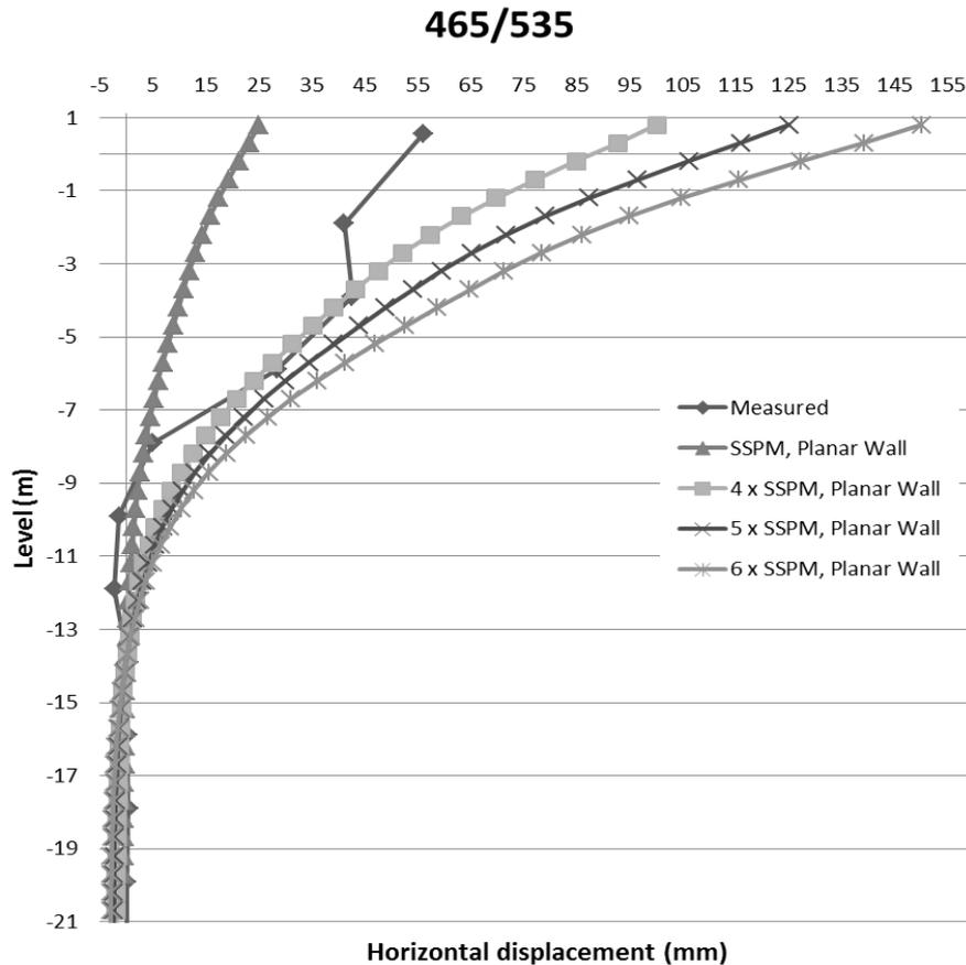
Figure 8.10 Measured and calculated horizontal displacements in section 465/535.
