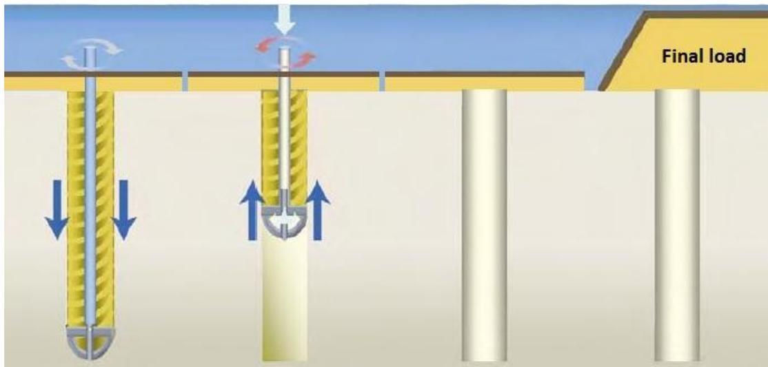
Figure 2.2 Production procedure of LC-columns (Keller ground engineering, 2008, modified).
