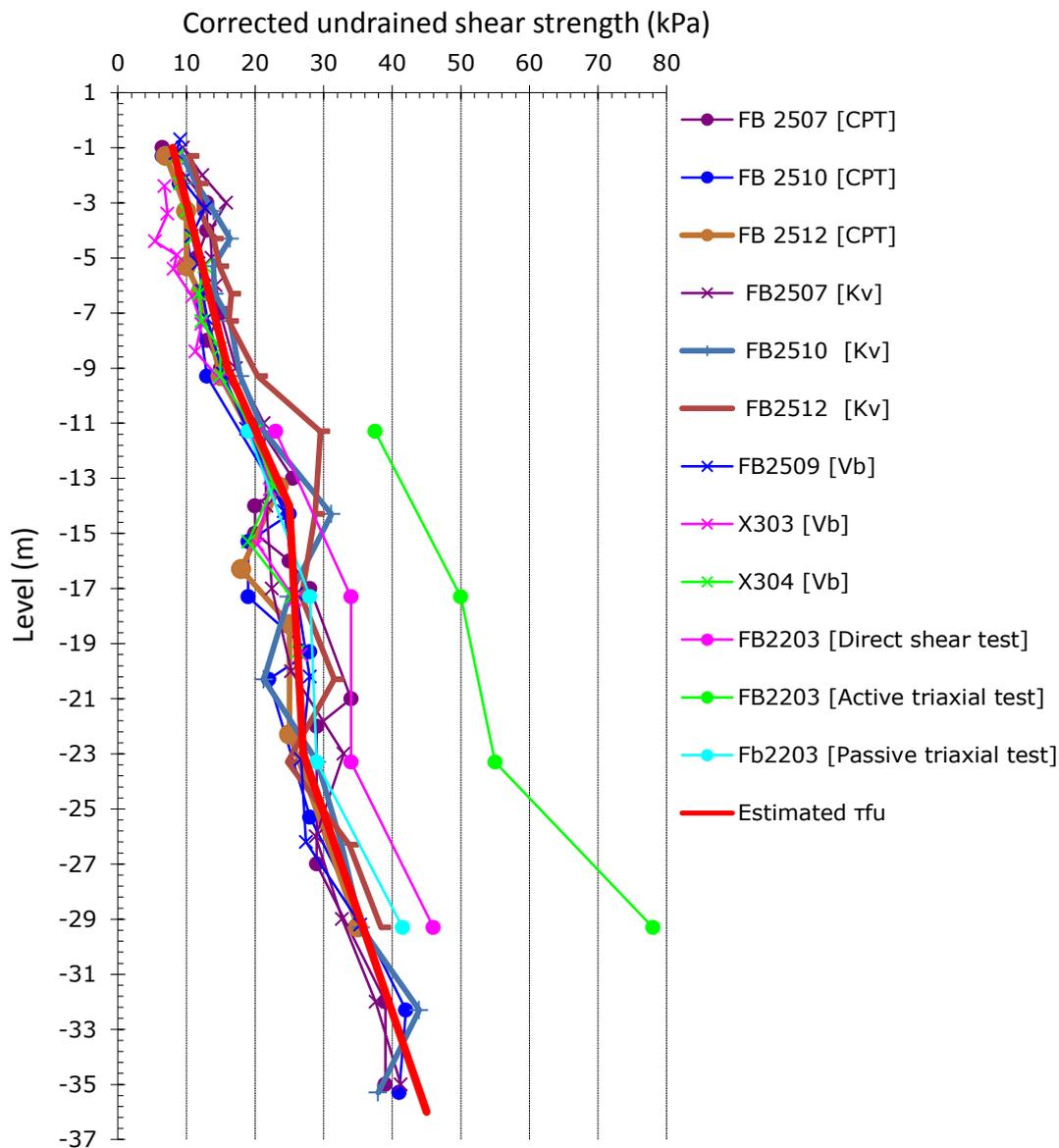
Figure 5.5 Corrected undrained shear strengths from tests made in the area and the estimated undrained shear strength is symbolised by a red line.
