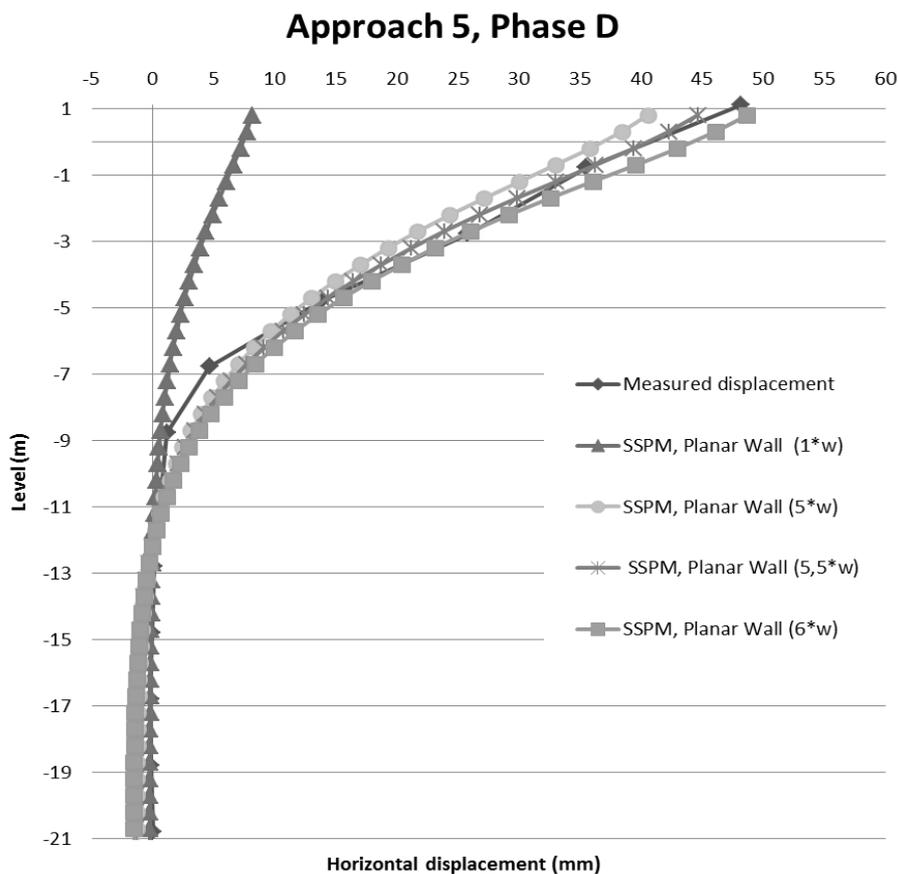
Figure 8.9 Horizontal displacement for Approach 5.
