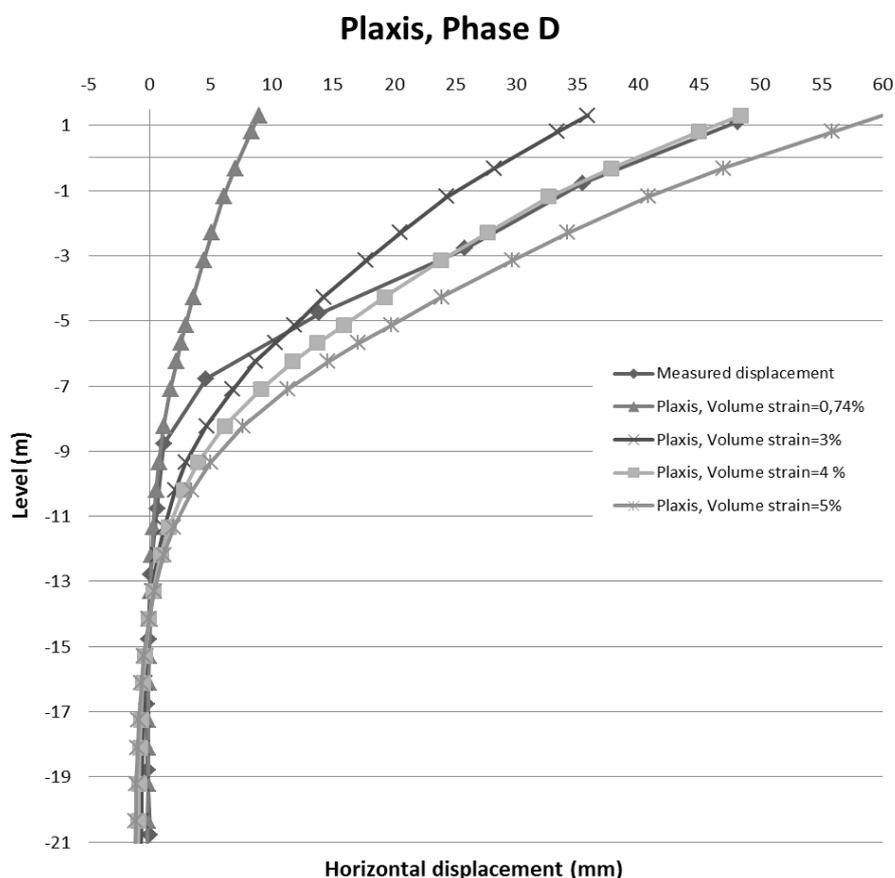
Figure 9.4 Horizontal displacement at the inclinometer position when the volume strain is varied compared to the measured displacement in section 465/300.
