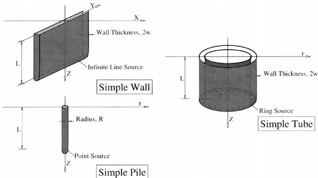
Figure 4.4 The geometries and notations used in the SSPM analysis (Sagaseta & Whittle, 2001).
