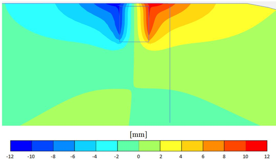
*Figure 9.2 View of the horizontal displacements that occur when the LC-column wall is applied with a volume strain of 0.74 % in PLAXIS.*
