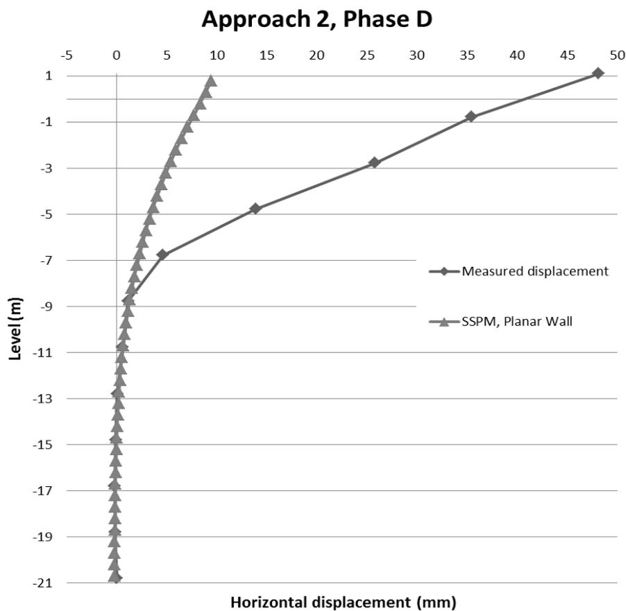
Figure 8.6 Horizontal displacements in Phase D, Approach 2.
