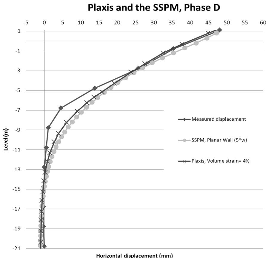
Figure 9.5 Results from PLAXIS compared to results with the SSPM for a planar wall in Approach 3.
