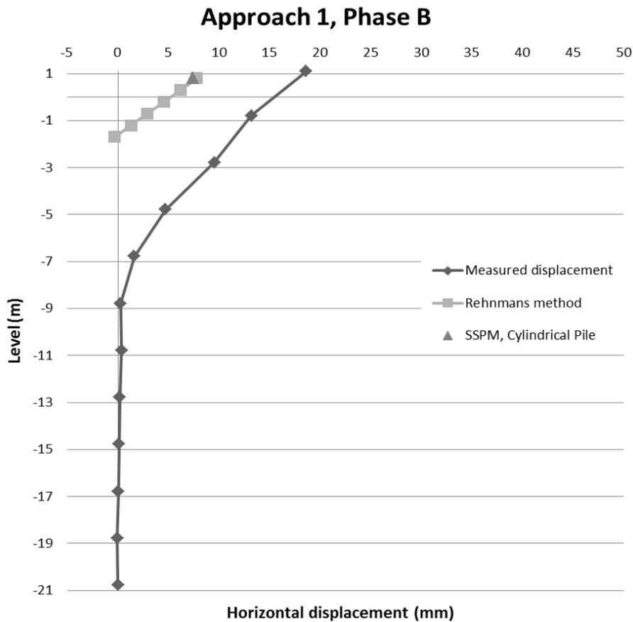
Figure 8.2 Horizontal displacements for Phase B, Approach 1.
