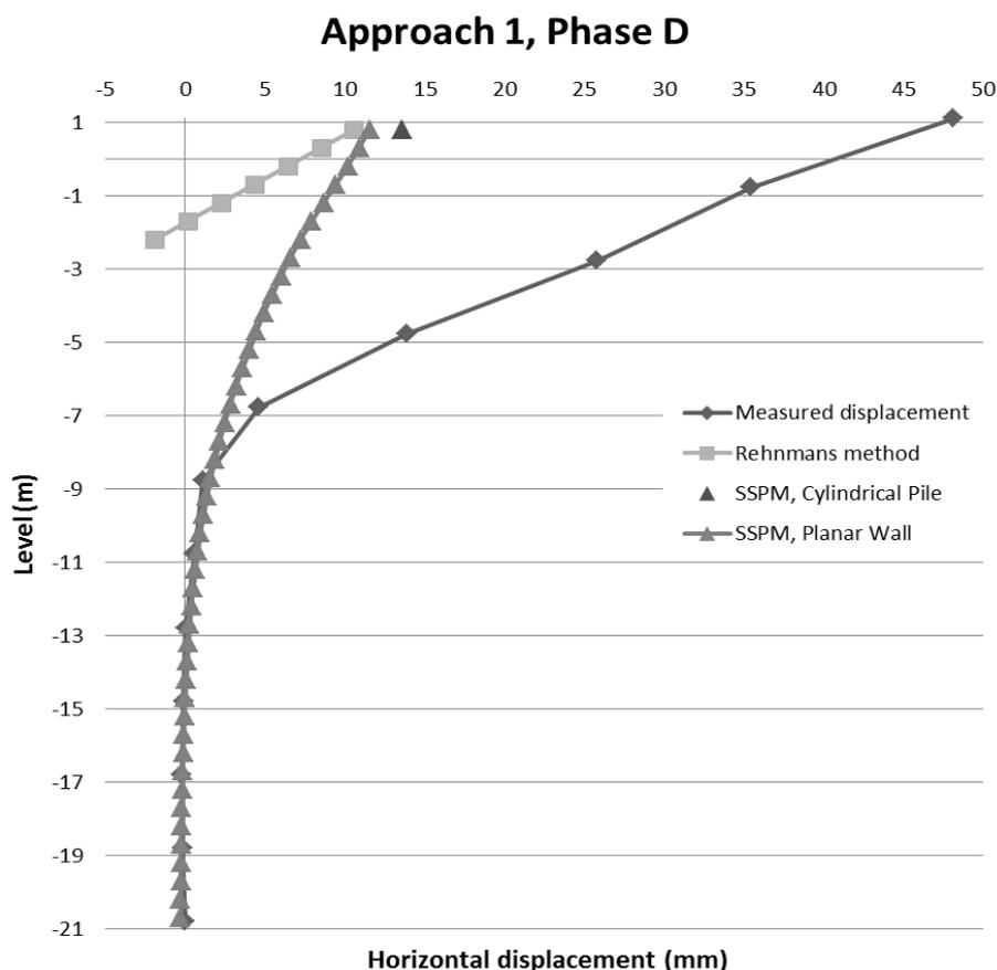
Figure 8.4 Horizontal displacements in Phase D, Approach 1.
