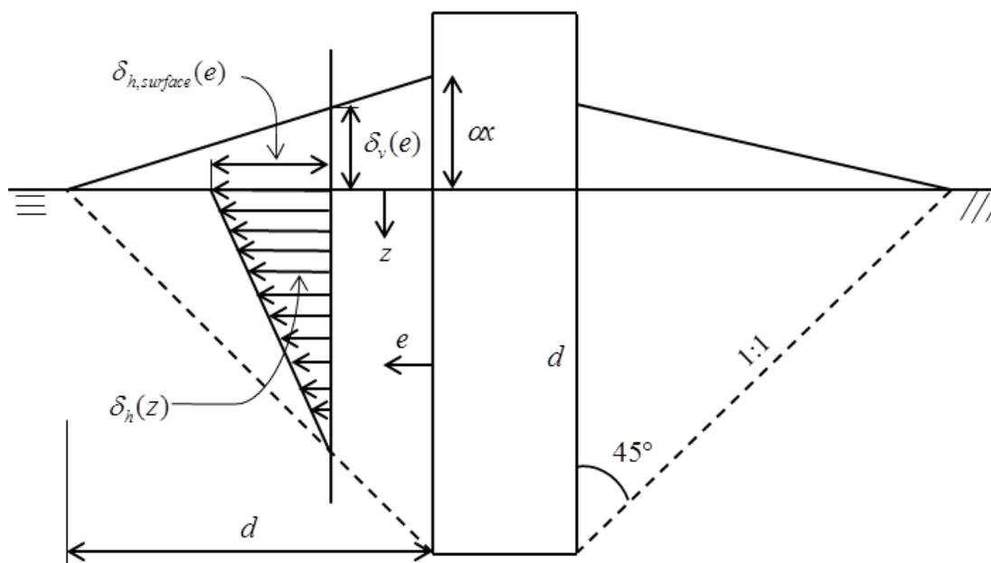
Figure 4.2 Ground surface heave and horizontal displacement distribution with the depth outside of the piling area (Hintze, S et al., 1997, modified)
