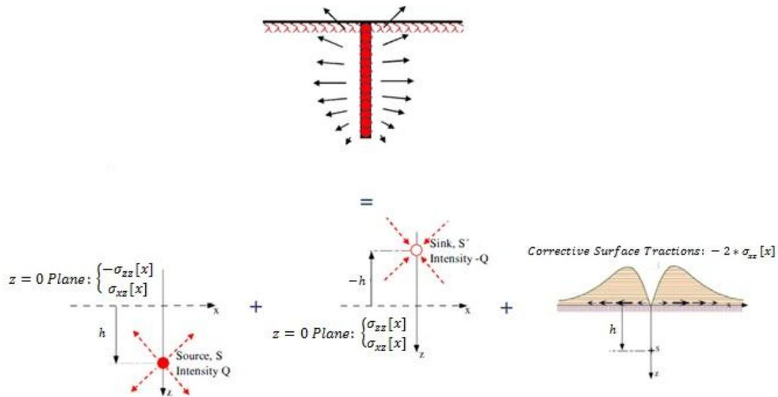
Figure 4.3 Steps included in the theory of the SSPM when estimating soil displacement due to piling, at the ground surface (Edstam, 2011).
