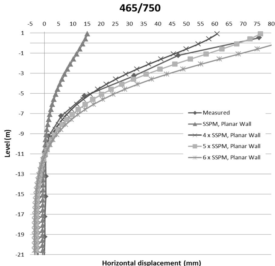
Figure 8.11 Measured and calculated horizontal displacements in section 465/750.
