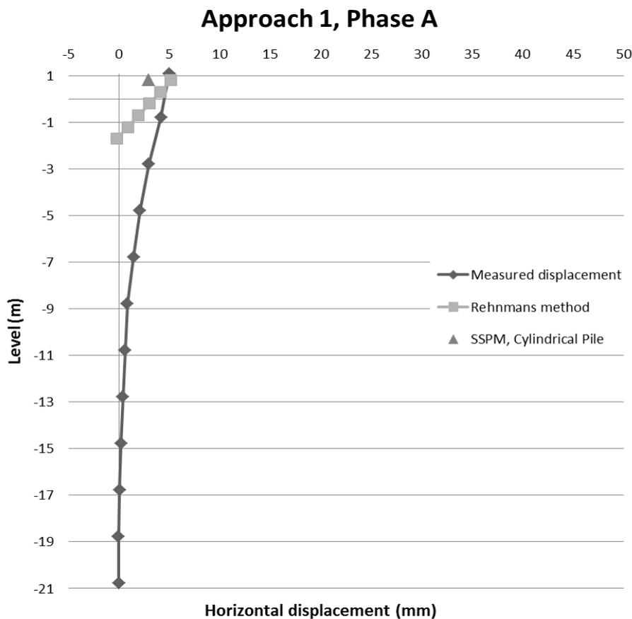
Figure 8.1 Horizontal displacements for Phase A, Approach 1.
