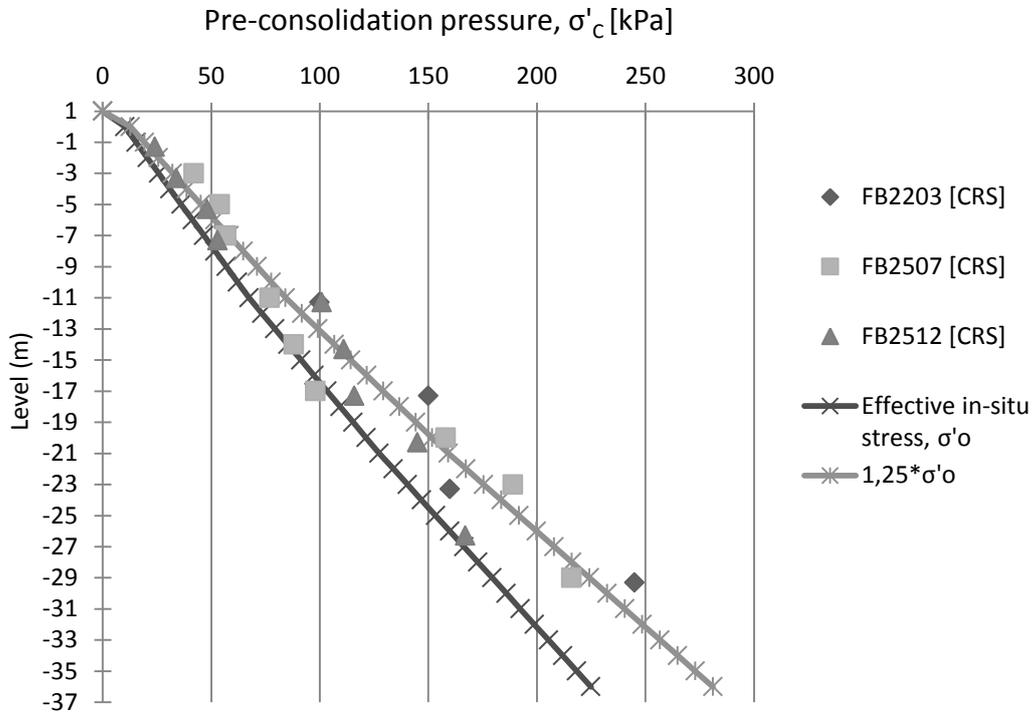
Figure 5.6 Plotted pre-consolidation pressures ( $\sigma'_c$ ) from CRS-tests, effective in situ stresses and a line  $1.25 * \sigma'_o$ .
