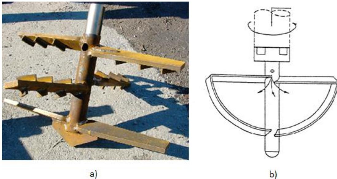
Figure 2.1 Mixing tools commonly used in Sweden. a) Pinnborr (LCM, 2002). b) SGF standard tool (SGF, 2000).
