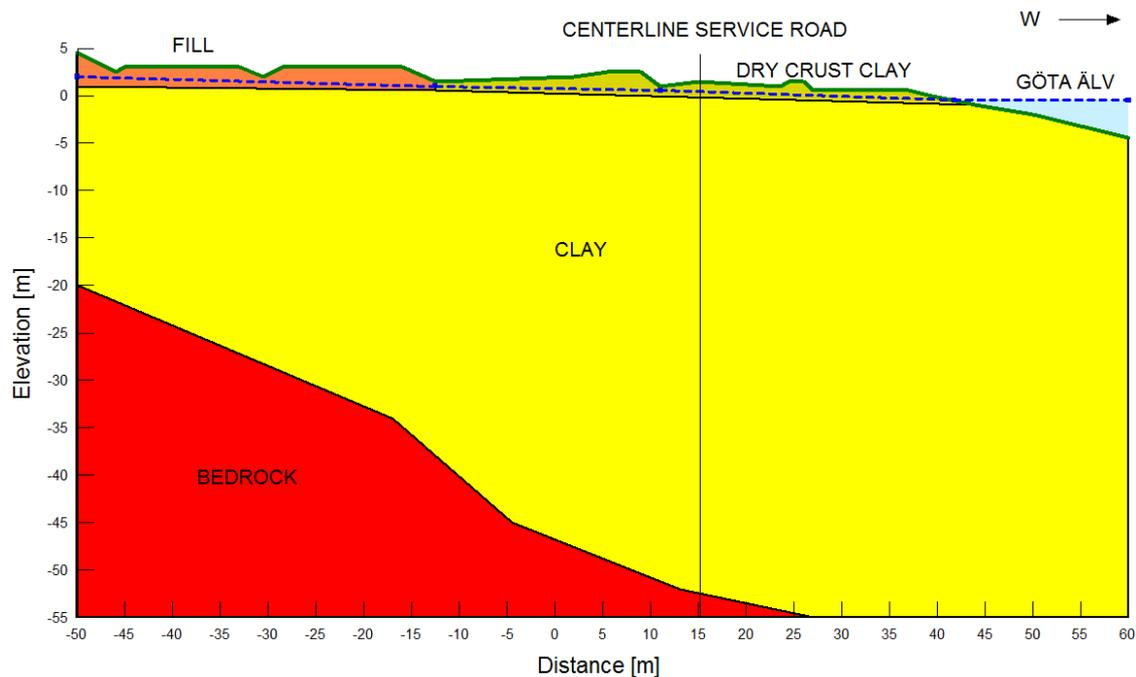
Figure 5.4 Estimated soil stratigraphy in section 465/300, the centerline of the constructed service road is marked.
