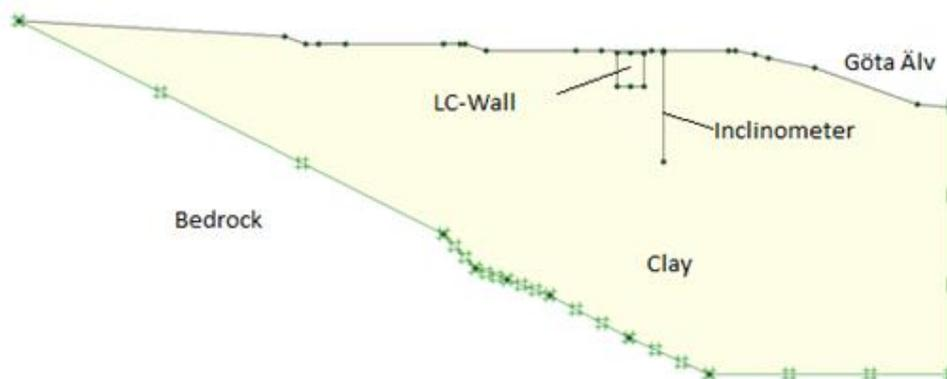
Figure 9.1 Overview of the PLAXIS model with boundaries, LC-column wall and inclinometer position.
