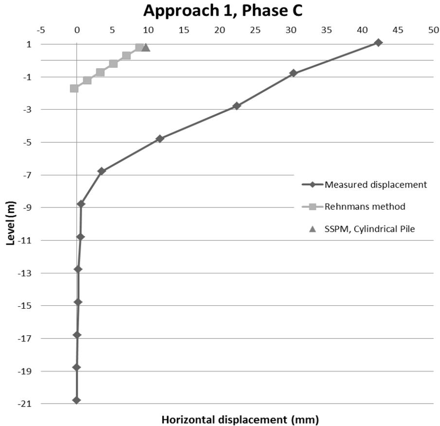
Figure 8.3 Horizontal displacements for Phase C, Approach 1.
