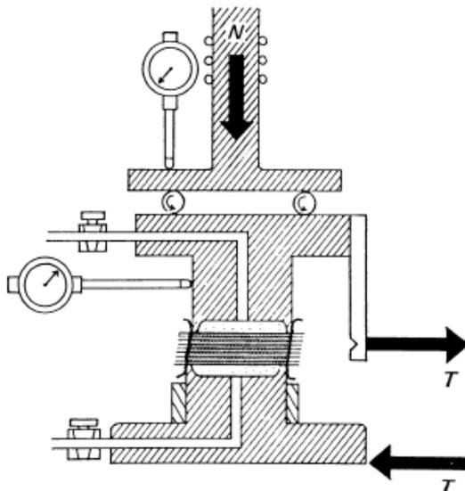
Figure 3.2 Principal sketch of a shear-apparatus (Larsson, 2008).
