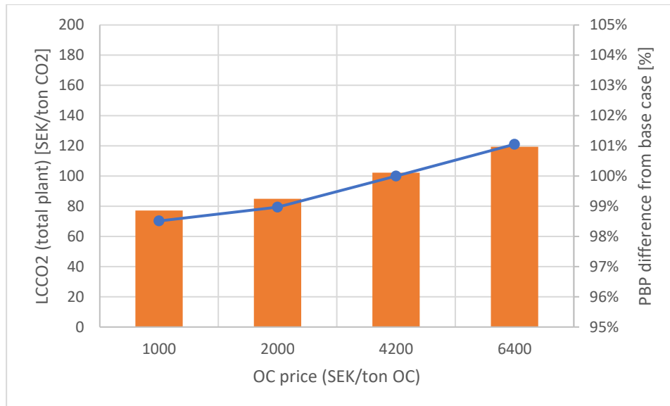
Figure 4.9. Impact of the OC price on the PBP (dots) and the break-even CO 2 cost (total plant) (columns)
