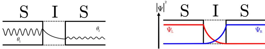
**Figure 2.3:** Schematics of a SIS junction. **(left)** The phase difference changes as wavefunction of the Cooper pairs tunnel through the junction. **(right)** The Cooper-pair density distribution around the junction.
