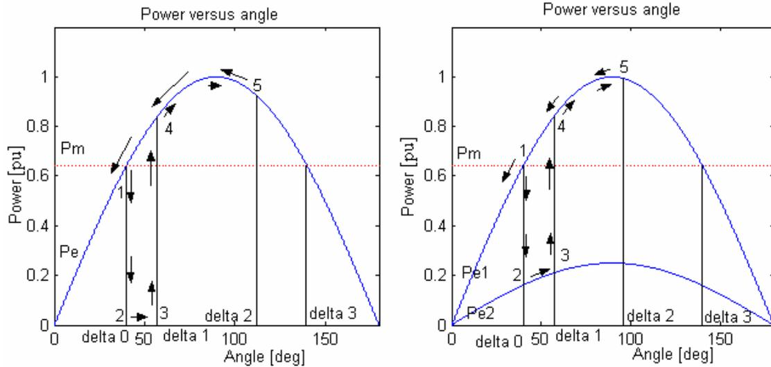
**Figure 2-4: Power transfer before, during and after a fault close to the turbine-generator**
