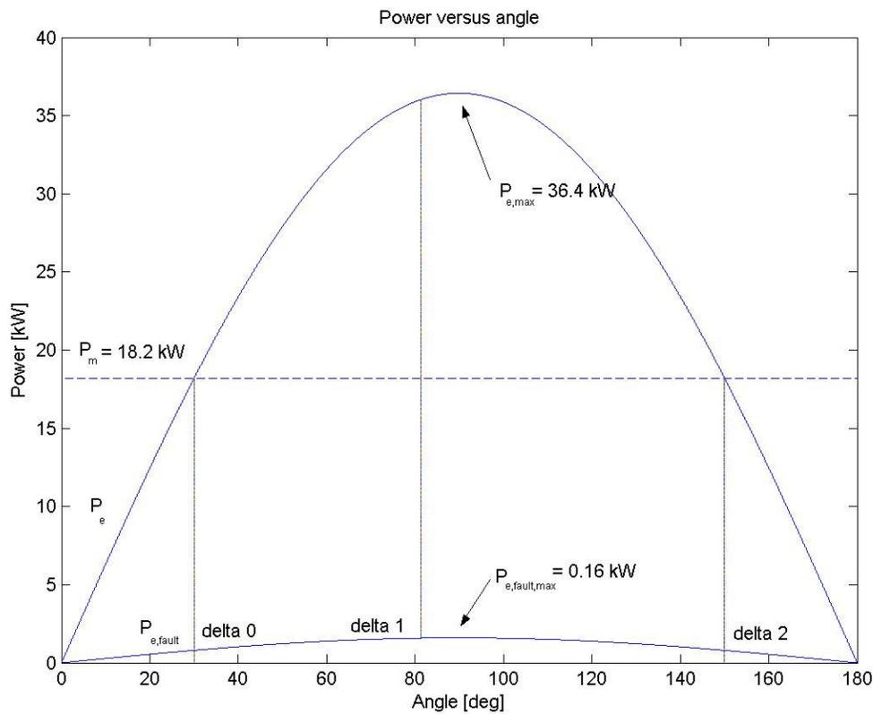
Figure 3-5: Input (dashed) and output (solid) power
