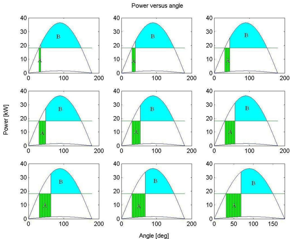
Figure 3-12: Riemann integration for equal-area criterion
