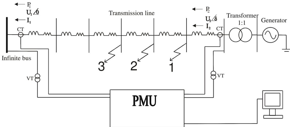
Figure 3-14: Lab setup with fault at three different locations
