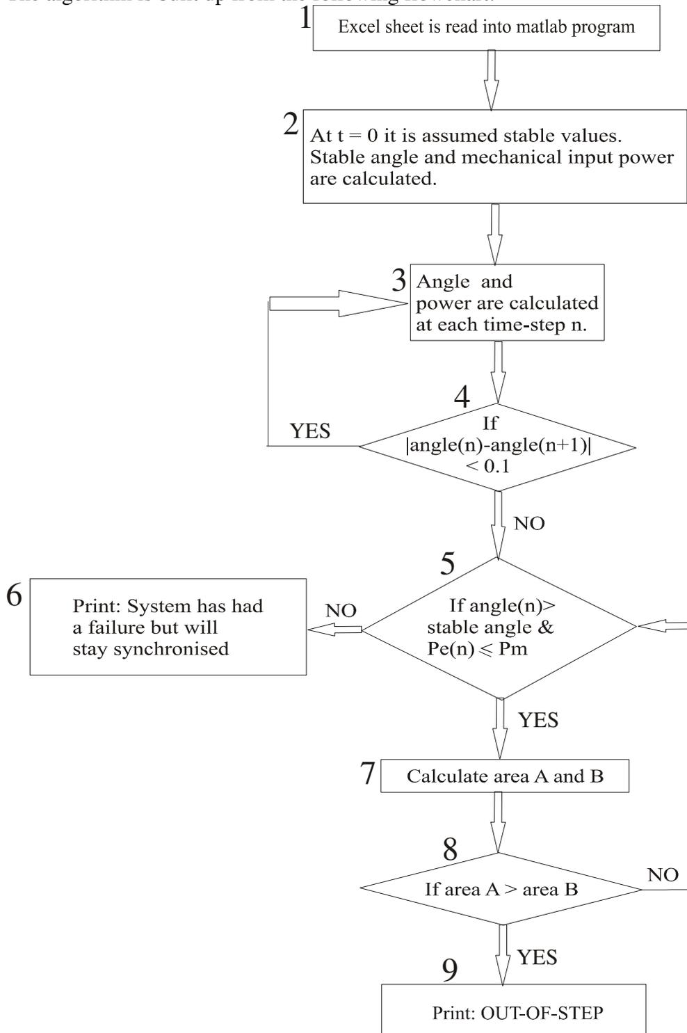
Figure 3-7: Flowchart of algorithm
