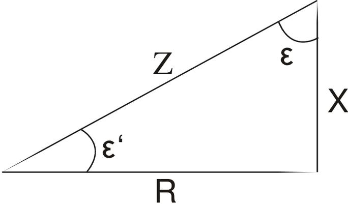
**Figure A-2: Impedance angle and loss angel**
