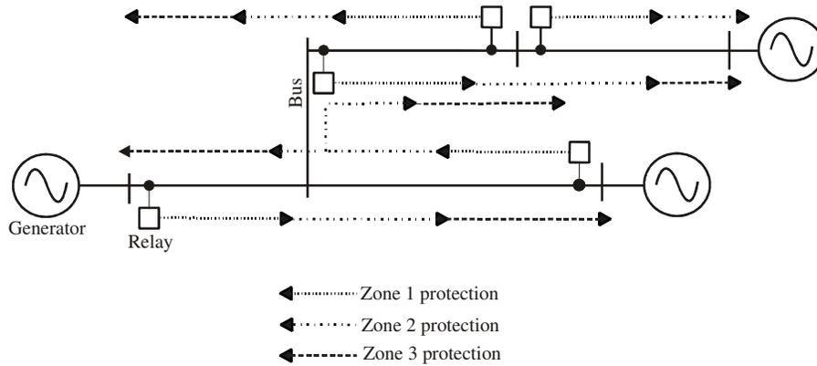
**Figure 2-9: Protection zones of a transmission line**
