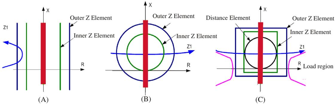
**Figure 2-10: Different power swing protection schemes**
