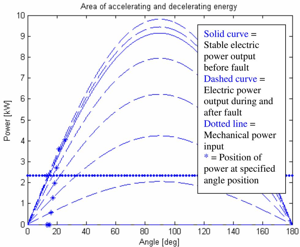
Figure 3-17: Power and angle variations during and after a fault.
