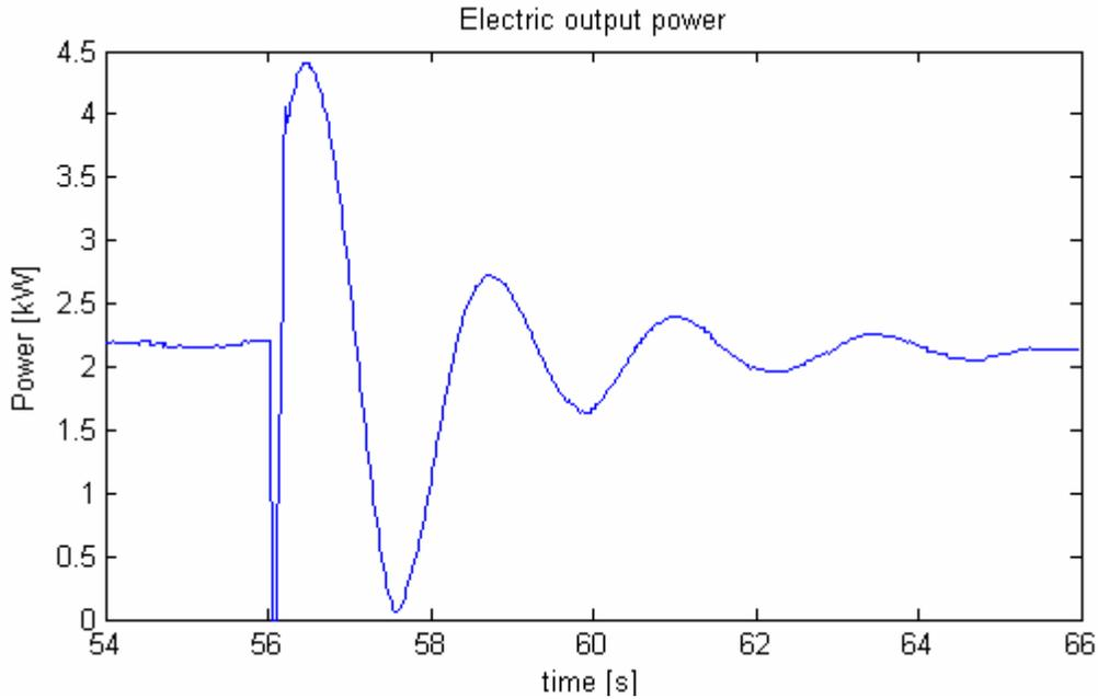
Figure 3-16: Electric output power at the selected fault position  $t = 56$  s
