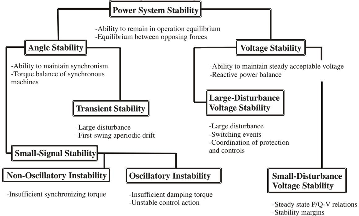
Figure 2-1: Schematic classification of power system stability
