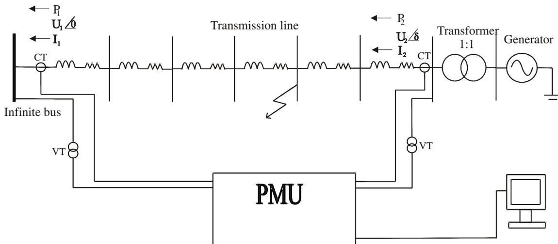
Figure 3-1: The power system model of the laboratory setup
