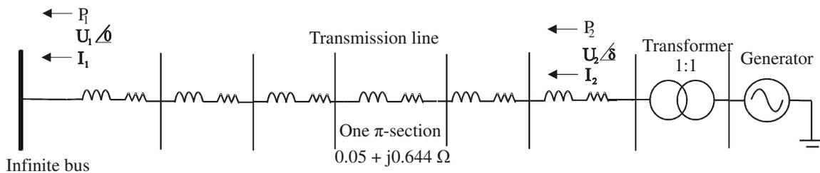
Figure 3-4: Single phase diagram
