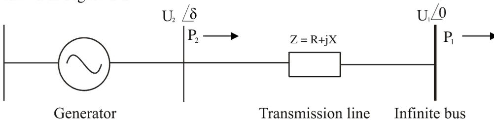
Figure 2-2: One machine against infinite bus diagram
