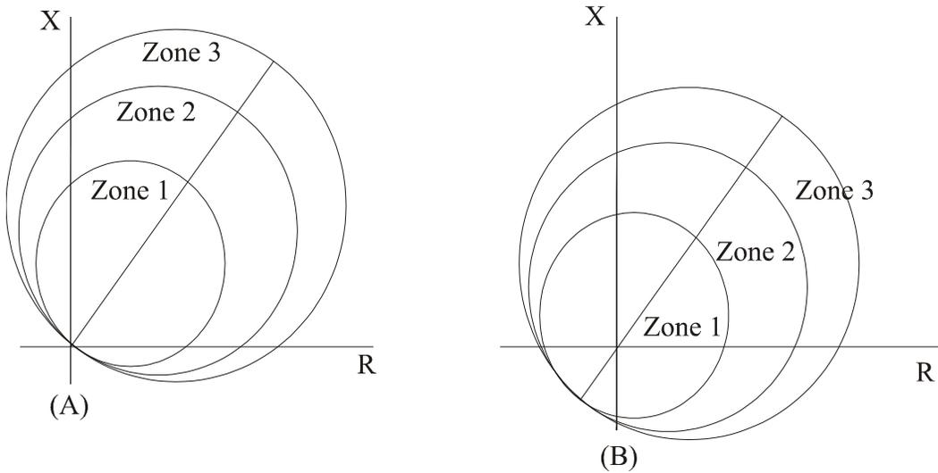
**Figure 2-8: Mho and offset mho characteristics**
