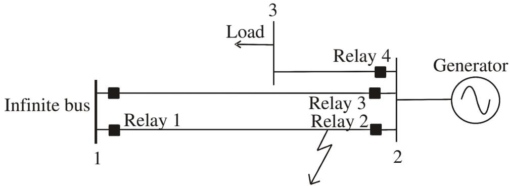
Figure 3-22: Fault in a larger network
