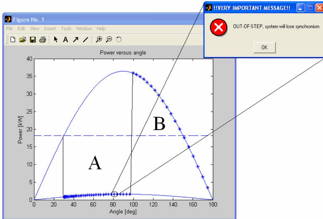
**Figure 3-21: Fault is cleared after the critical fault clearing time**
