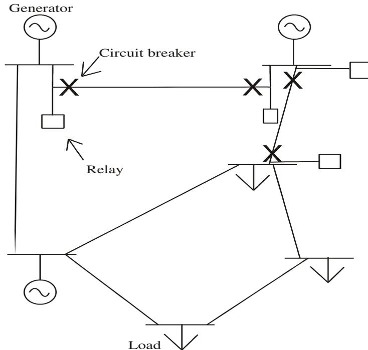
Figure 2-6: Meshed power system
