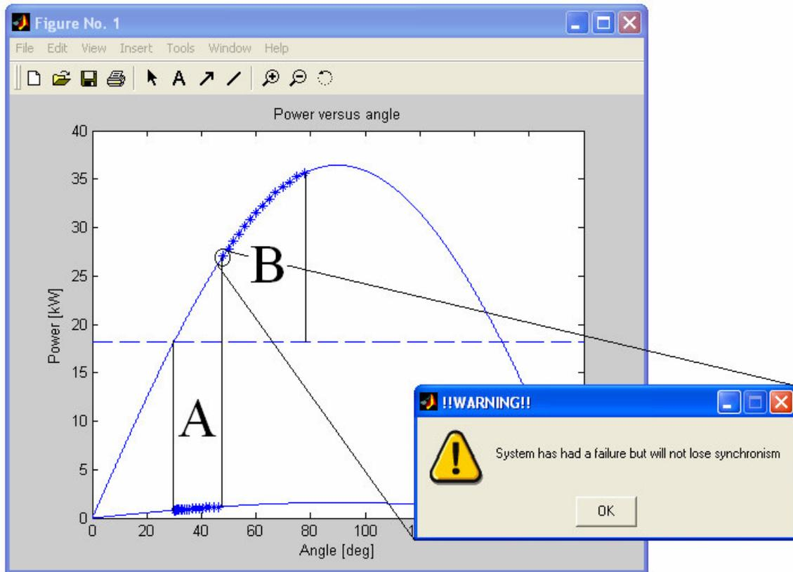
**Figure 3-20: Fault is cleared before the critical fault clearing time**
