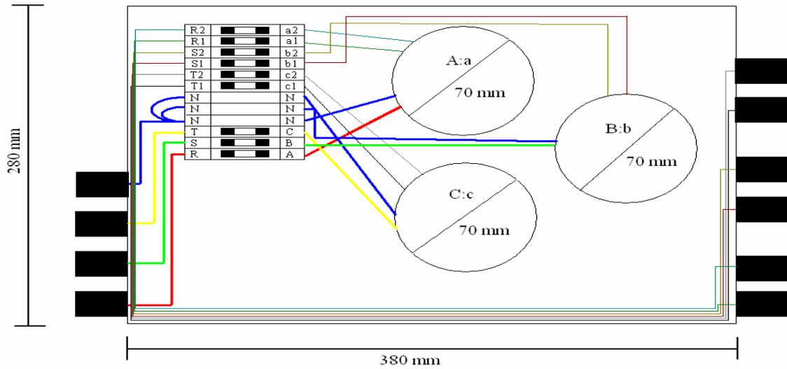
**Figure C-1: Connection diagram of a three phase instrument transformer**
