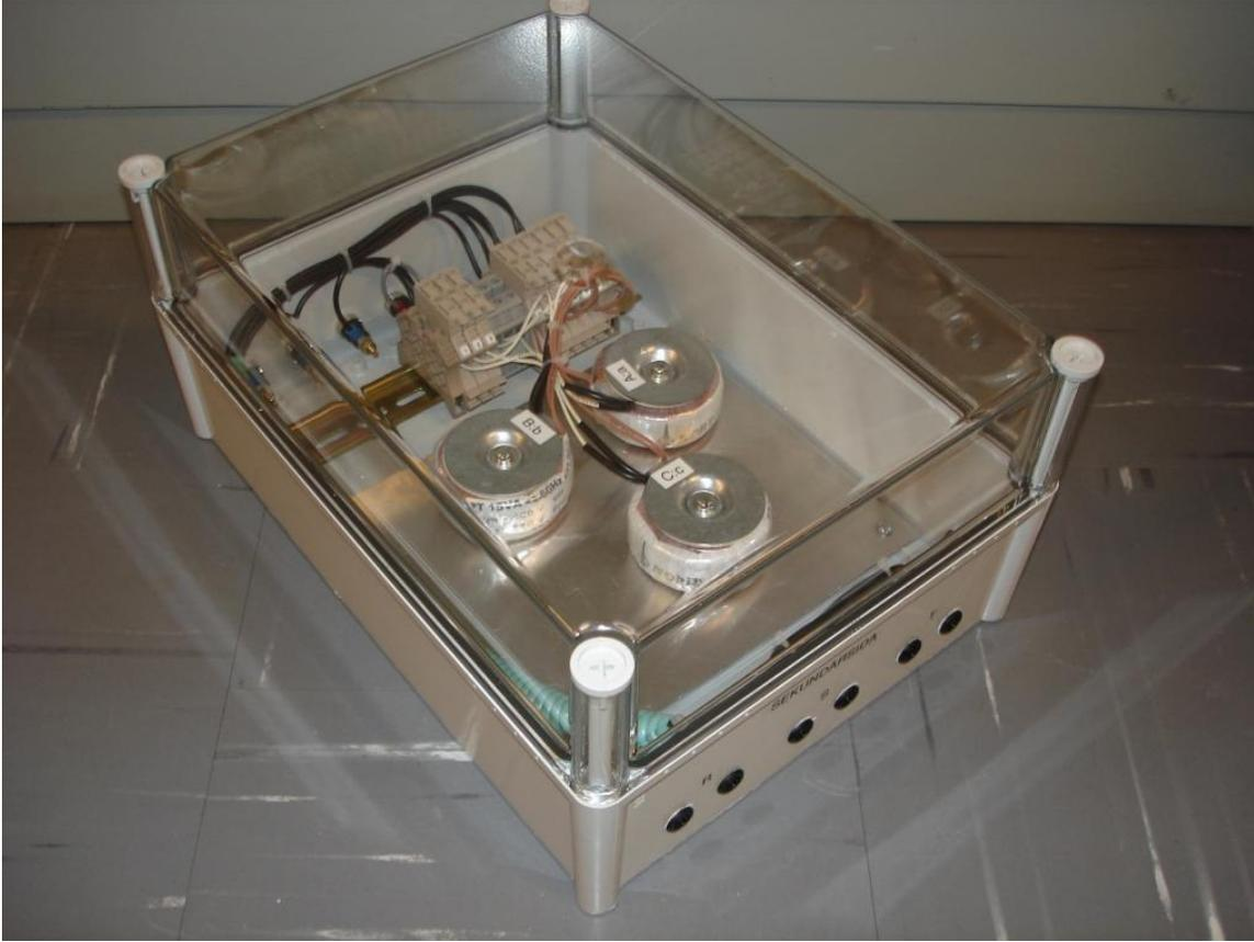
**Figure C-2: Voltage instrument transformer**
