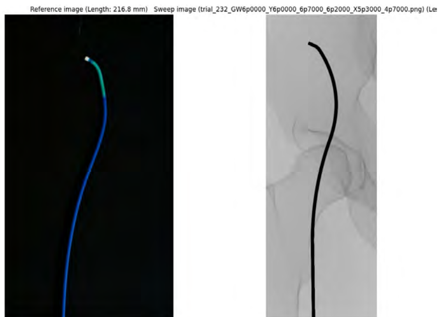
Figure 5.8: Real and simulated images used for comparison of the JR4 8F guiding catheter from Medtronic and an accompanying thin and stiff guidewire.
