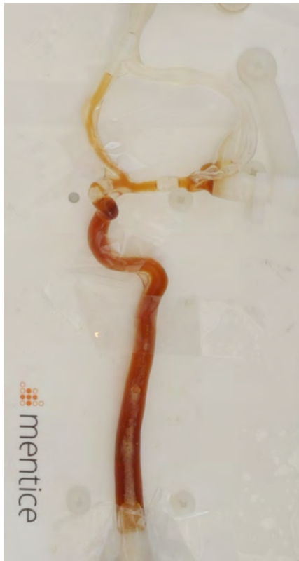
(a) Physical SIM phantom. Injected with coffee to highlight the vessel structure.
