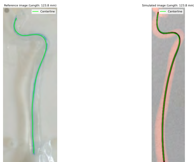
Figure 5.6: Resulting images of a microcatheter in the physical SIM environment and the VIST simulation system, together with their corresponding extracted centerlines.
