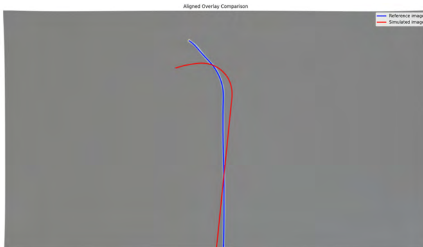
Figure 5.15: Aligned overlay comparison of the centerlines extracted from the real and simulated images of the XBLAD 4 8F guiding catheter from Cordis and the accompanying thick and stiff guidewire.
