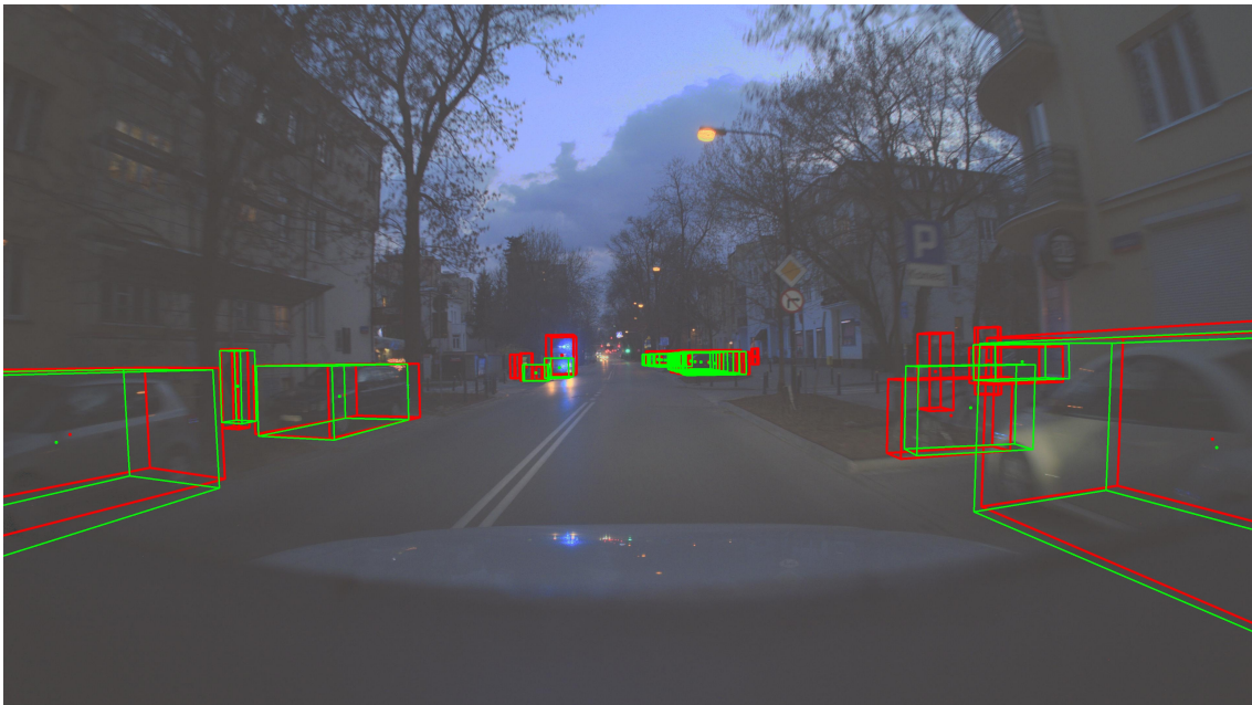
Figure 5.2: Example image from the validation split of the ZOD dataset. Red boxes are the ground truth labels and green boxes are predictions by the baseline model.
