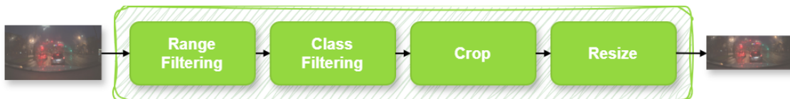
Figure 3.1: Overview of the image transformation pipeline applied to each input frame before training. This includes range filtering, class filtering, cropping, and resizing.
