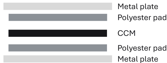
Figure 4.29: Set-up for CCM assembly using polyester pad and metal plate.
