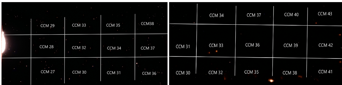
Figure 4.6: Illustration of areas used from the cathode (left) and anode (right) during the assembly and their corresponding CCM.
