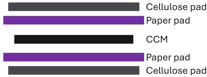
Figure 4.32: Set-up for CCM assembly using non-residual paper as sandwich material under the cellulose pad.
