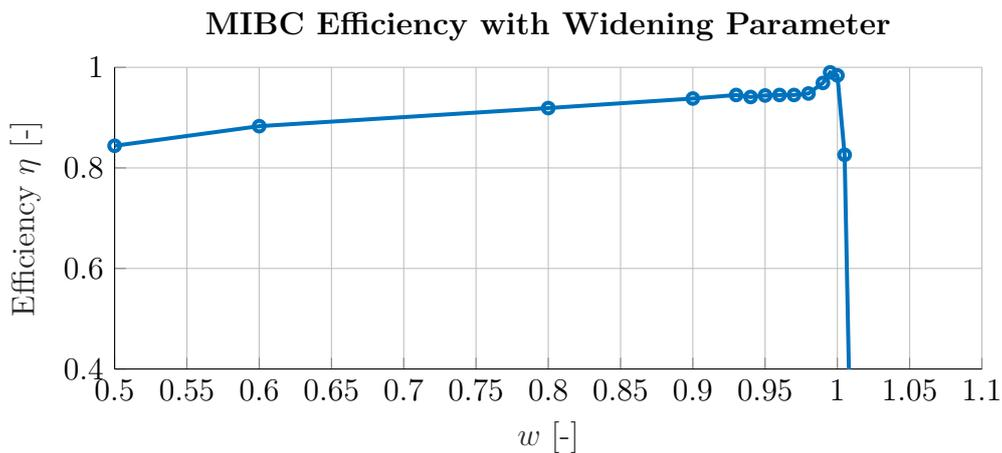
**Figure 4.13:** The impact on efficiency of making the OFF-state of the low side transistors shorter ( $w > 1.00$ ) or longer ( $w < 1.00$ ).
