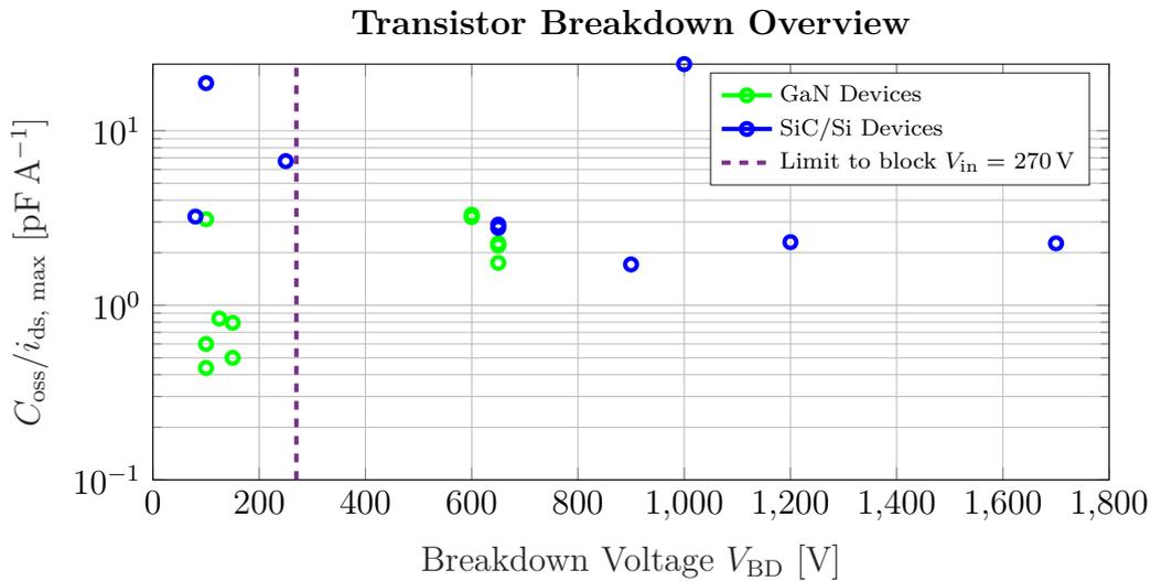
**Figure 2.1:** The ratio  $C_{\text{oss}}/i_{\text{ds, max}}$  for different commercial devices in GaN, Si, and SiC for the respective rated breakdown voltage of each device. More details are available in Appendix A.
