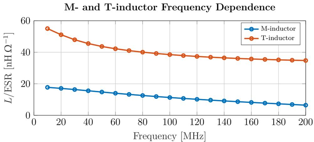
**Figure 5.5:** The frequency dependence of the  $L/ESR$ -ratio for an M- and T-inductor respectively both featuring approximately 220 nH at 50 MHz.
