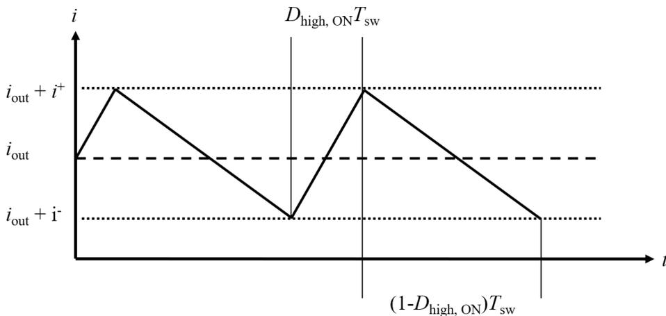
**Figure 3.6:** Schematic graph of the inductor current over time, in continuous mode the current oscillates between  $i_{out} + i^-$  and  $i_{out} + i^+$  while the output current of the converter is the average,  $i_{out}$ .
