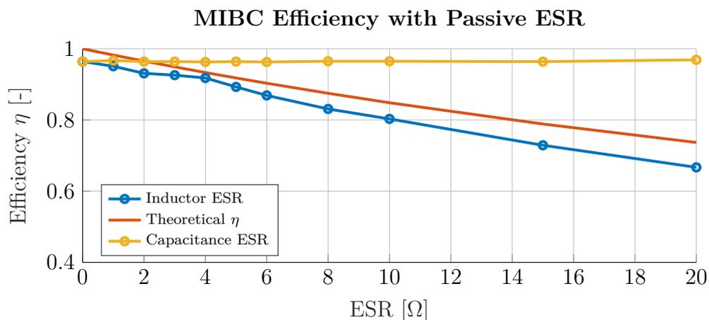
**Figure 4.14:** Efficiency degradation of the MIBC as the ESR of the flywheel inductors and capacitor is increased. To compensate a decreasing  $V_{\text{out}}$  the duty cycle is tuned to always provide  $\approx 28$  V delivered at the output of the converter.
