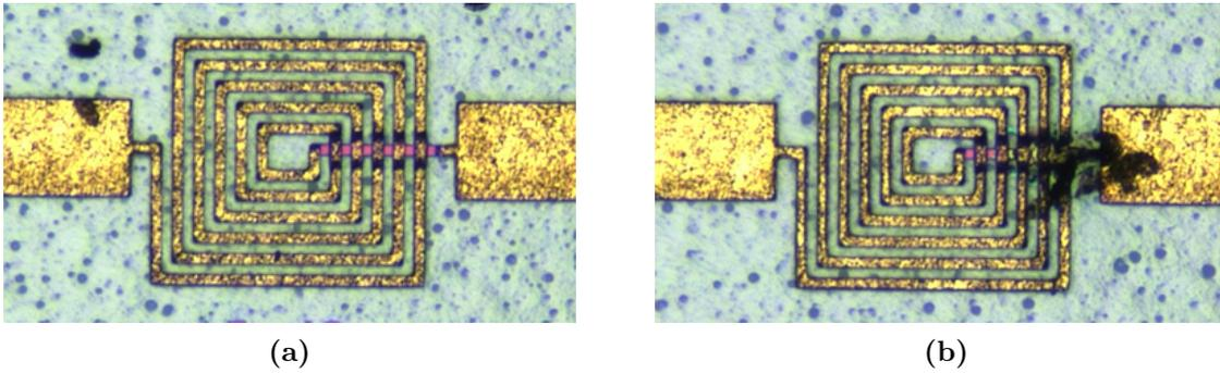
**Figure 5.12:** Images showing the same S-inductor design (6 turns standard), where (a) is in working condition and (b) has fused after a high current was supplied.
