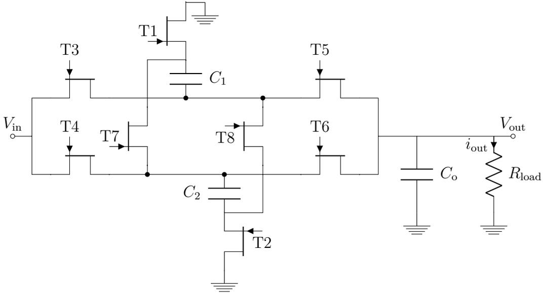
**Figure 3.2:** Series-parallel switched capacitor converter capable of a fixed VSDR of 2. By operating T1-T8 with different control schemes (from Table 3.1) conversion ratios of 1-to-1 and 1-to-2 are also possible.
