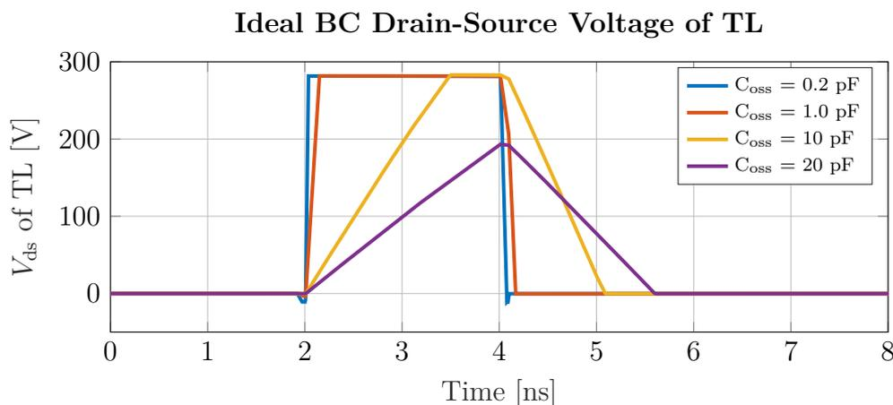
**Figure 4.4:** Drain-source voltage across the high side transistor for different values of the output capacitance at steady state ( $t + 10 \mu s$ ).
