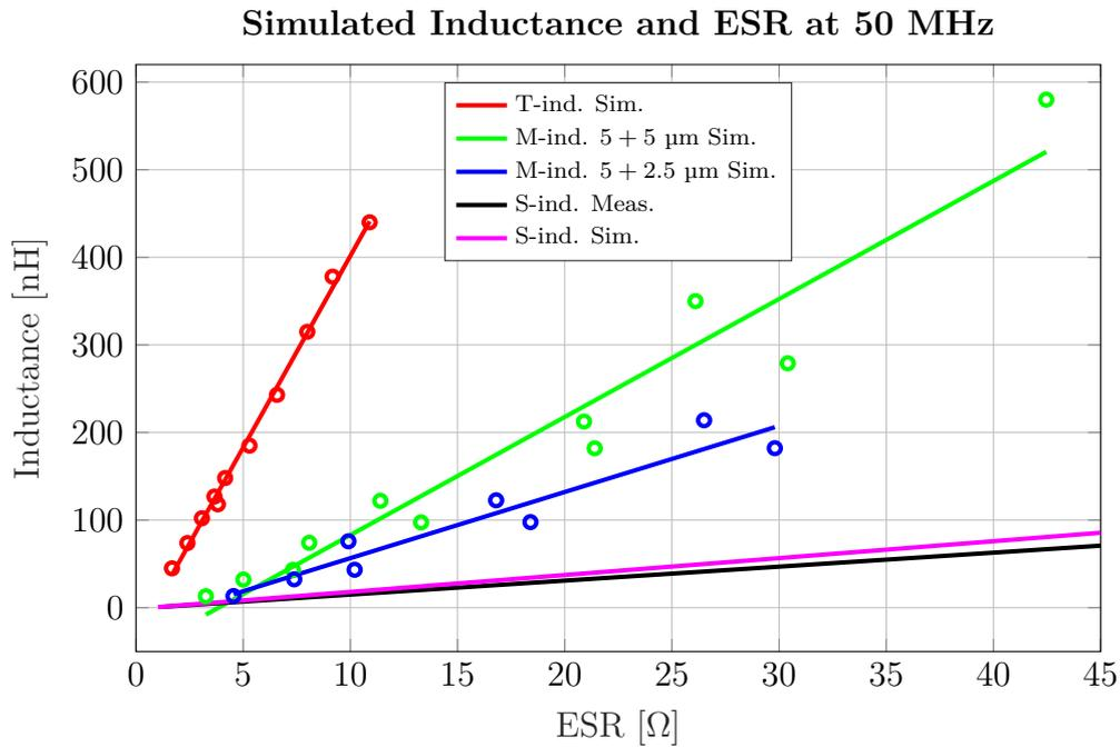
**Figure 5.4:** The simulated and measured inductance as a function of the ESR for T-, M-, and S-inductors with different conductor separations. Circles represent ADS FEM-simulation and the lines are fitted linear functions for each inductor type.
