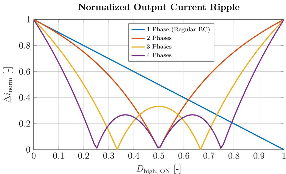
**Figure 3.9:** The normalized output ripple current from (3.19) as a function of the duty cycle for a conventional Buck converter and interleaved converters with 2, 3 or 4 phases.
