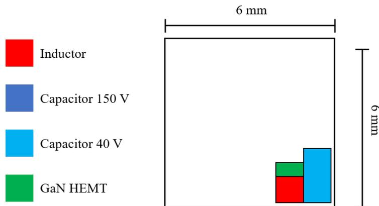
**Figure 6.3:** A schematic drawing of the space requirements for each component type in the suggested integrated Buck converter using the M-technology.
