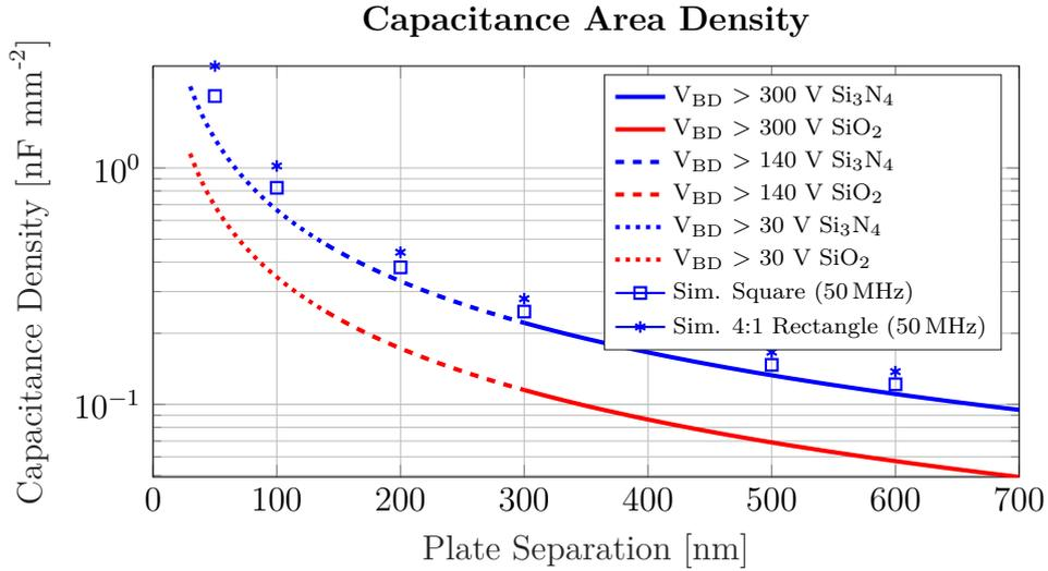
**Figure 5.13:** The capacitance density obtainable with  $\text{SiO}_2$  or  $\text{Si}_3\text{N}_4$  as dielectric media as a function of the plate separation  $d$  and the breakdown voltage  $V_{BD}$ . Results both from theory and FEM simulations at 50 MHz.
