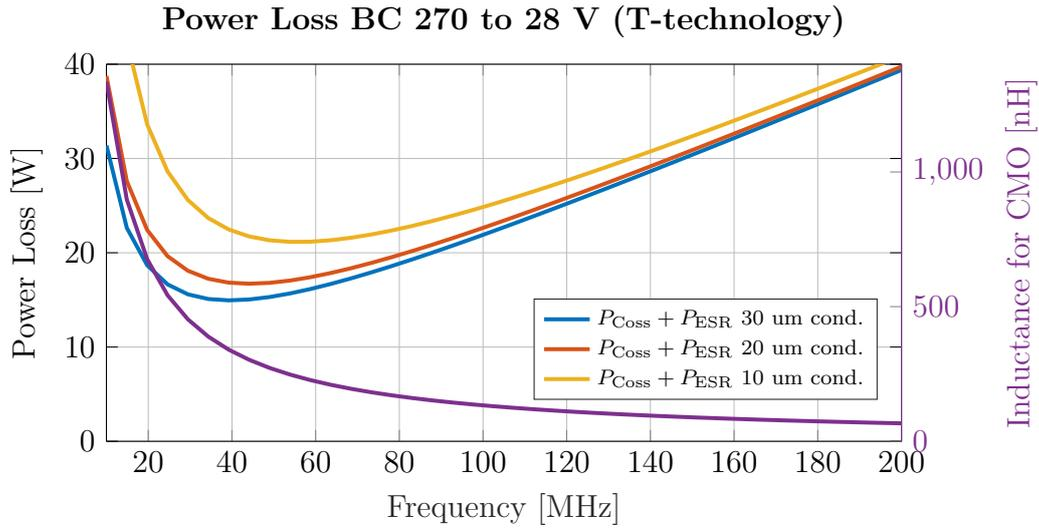
**Figure 6.4:** The sum of the loss terms together with the required inductance for CMO at 26.3 W output power in the T-technology.
