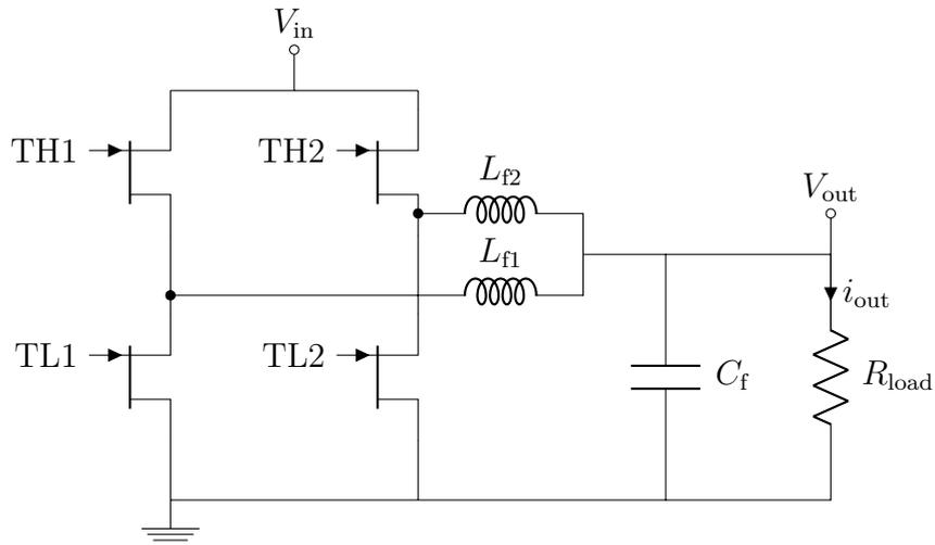
**Figure 3.8:** Principle design of an  $N = 2$  IBC, the transistor pairs are driven  $180^\circ$  out of phase.
