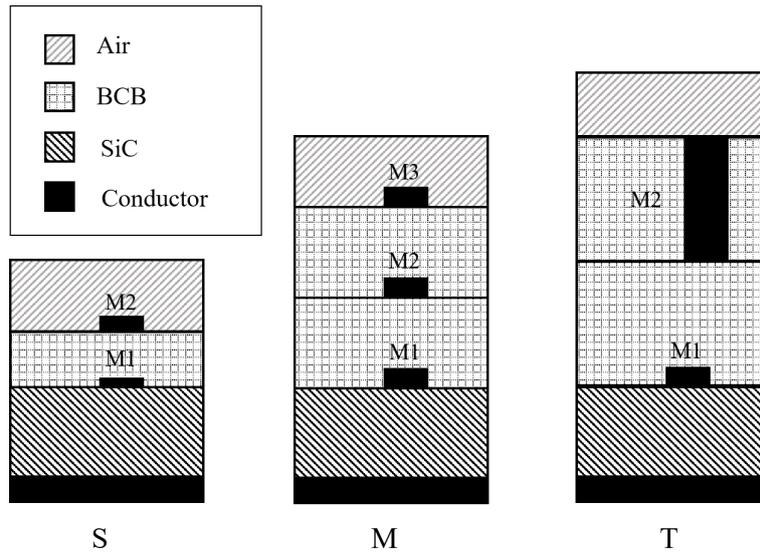
**Figure 5.1:** Overview of the S-, M-, and T-type technology realized with the Chalmers In-House GaN technology and the BCB back-end under development (not to scale).
