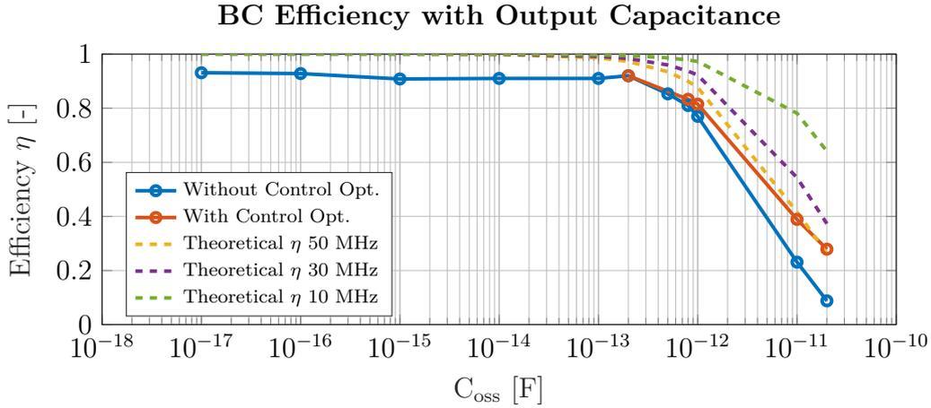
**Figure 4.5:** The efficiency of the simulated Buck Converter operating at 50 MHz for different output capacitance values, together with the efficiency  $\eta$  as suggested by the design equations for a selection of switching frequencies.
