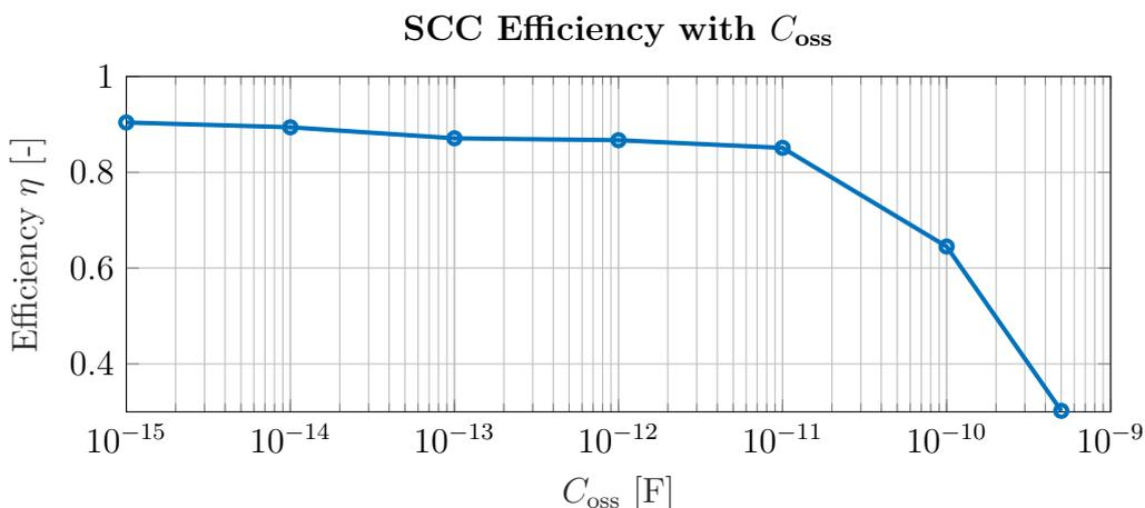
**Figure 4.17:** Efficiency decrease as  $C_{oss}$  increases for the SCC topology operating at 400 kHz with  $C_1 = C_2 = 5$  nF.
