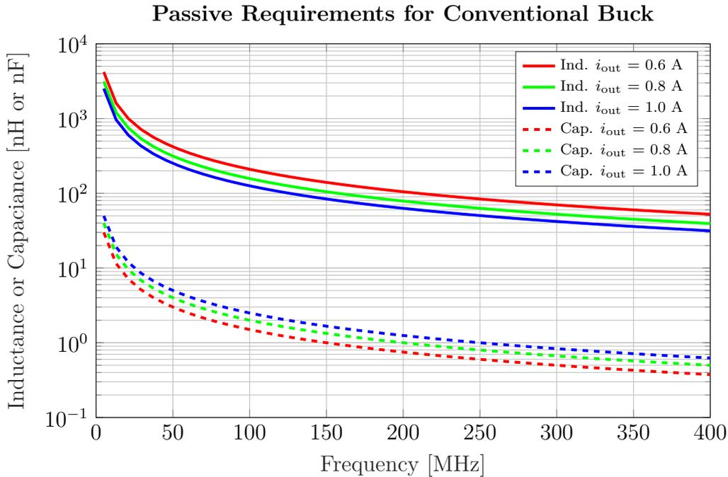
**Figure 3.7:** The component values for the flywheel inductor  $L_f$  and capacitor  $C_f$  as a function of switching frequency, for an ideal, 270 to 28 V, Buck converter operating at an output current of 0.6, 0.8 and 1 A (19 W, 22 W and 28 W). The inductor current ripple is the limit for CMO and the voltage ripple is fixed at 1 V peak-to-peak.
