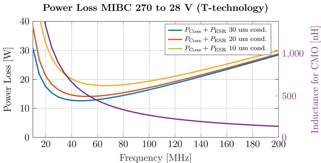
**Figure 6.8:** The power loss as a function of frequency for the MIBC topology with different conductor thicknesses in the T-inductors.
