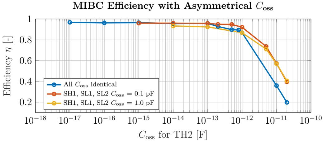
**Figure 4.12:** The efficiency of the MIBC once  $C_{oss}$  is both the same and not the same for the low voltage transistors (TH1, TL1, and TL2) and the high voltage transistors (TH2).
