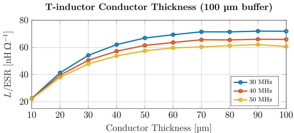
**Figure 5.9:** T-inductor performance for different conductor thicknesses (100 μm buffer).
