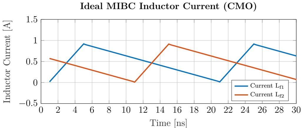
**Figure 4.9:** Flywheel inductor current through each branch of the MIBC for  $L_{f1} = L_{f2} = 500 \text{ nH}$  at steady state ( $t + 10 \mu\text{s}$ ). The converter is in CMO.
