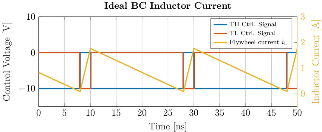
**Figure 4.2:** The simulated inductor flywheel current and control signals for the ideal BC at steady state ( $t + 10 \mu\text{s}$ ).
