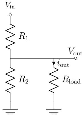
**Figure 3.1:** Schematic of the simplest DC-to-DC converter, the resistive voltage divider.
