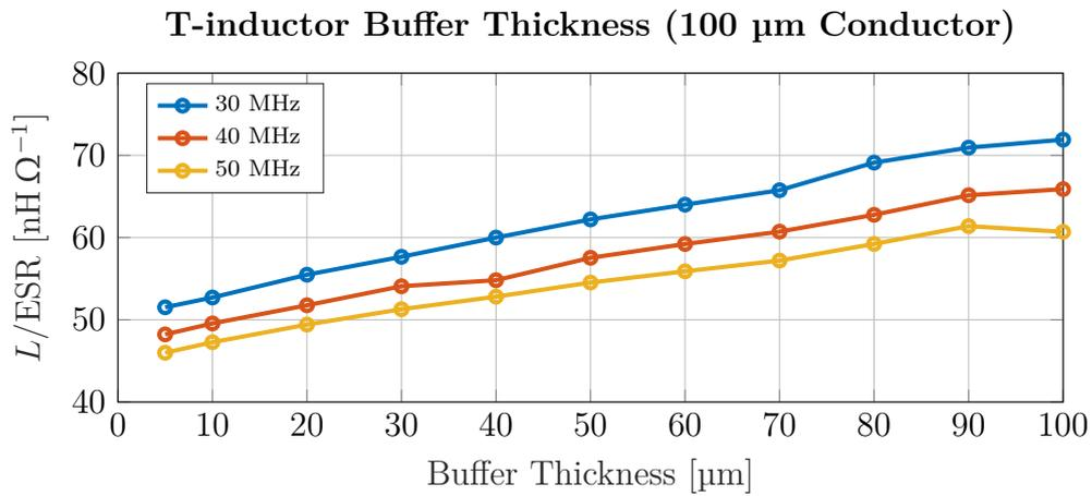
**Figure 5.8:** The impact of buffer thickness on the  $L/ESR$ -ratio for the T-inductors (100 μm conductor).
