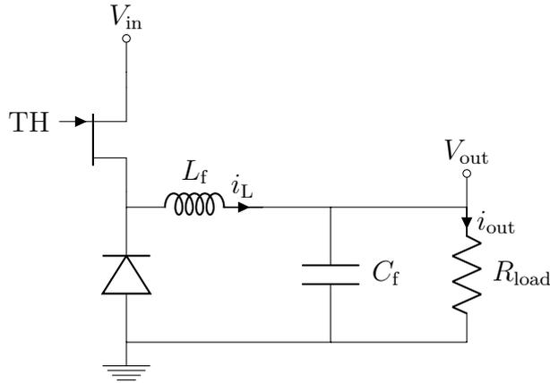
**Figure 3.4:** Schematic view of a nonsynchronous Buck converter, one control signal is supplied to transistor TH to switch between the ON and OFF state.
