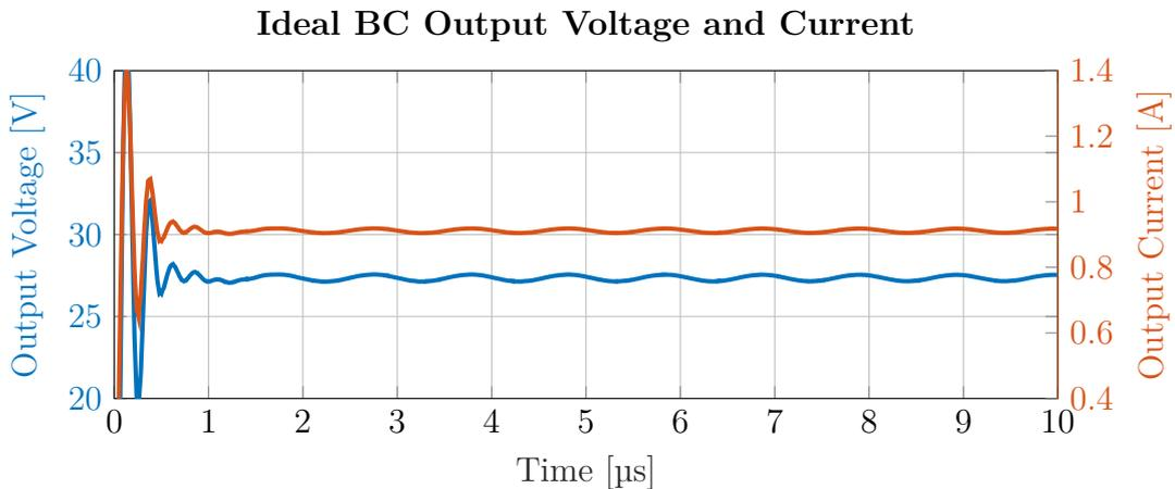
**Figure 4.1:** The simulated output voltage and current of an ideal 50 MHz BC.
