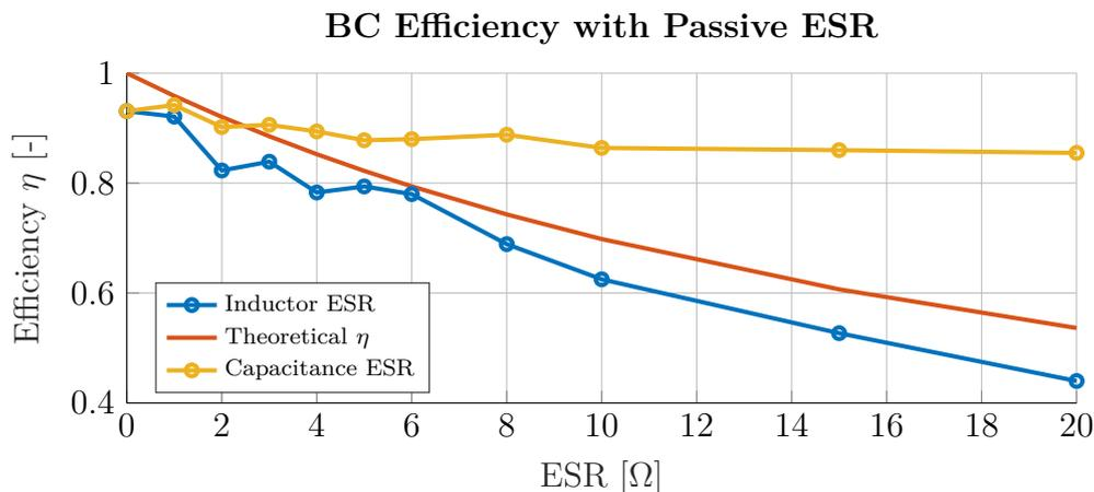
**Figure 4.7:** The efficiency of the BC with increasing ESR for the flywheel inductor and capacitor. The duty cycle  $D_{high, ON}$  has been increased to provide 28 V at the output for increasing  $L_f$  ESR.
