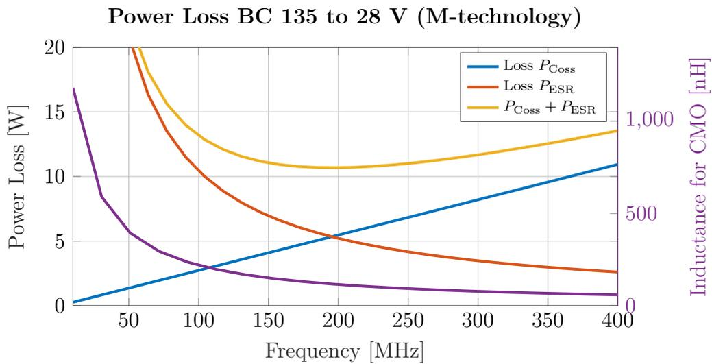
**Figure 6.10:** The most important loss factors for the  $135 \text{ V}$  to  $28 \text{ V}$  BC in the M-technology operating at an output of  $26.3 \text{ W}$ .
