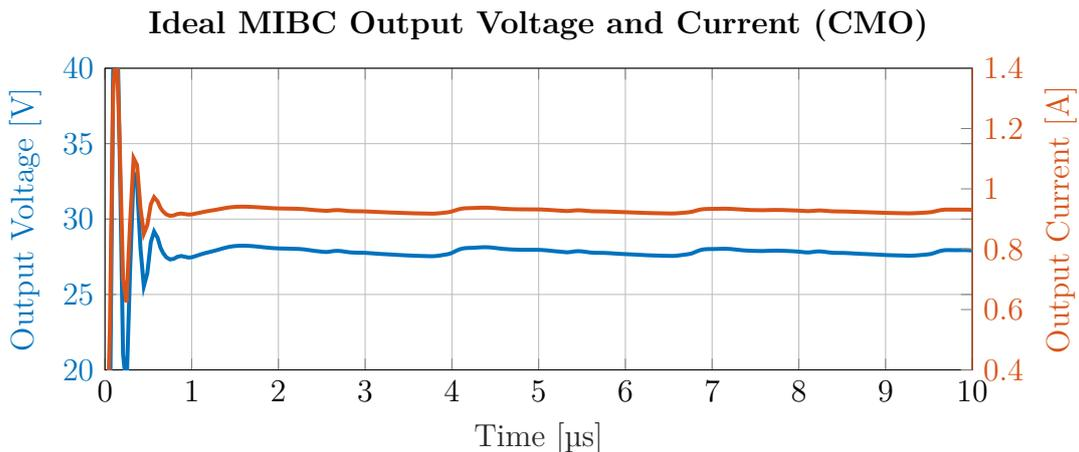
**Figure 4.10:** The output voltage and current as the MIBC reaches steady state.
