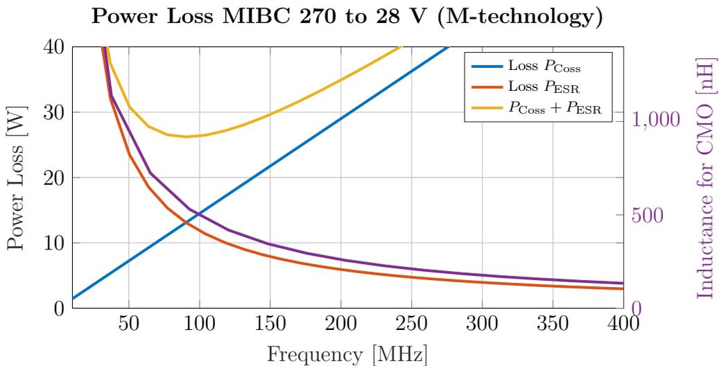
**Figure 6.6:** The power loss due to parasitic capacitance and inductor ESR for the MIBC realized with the M-technology.
