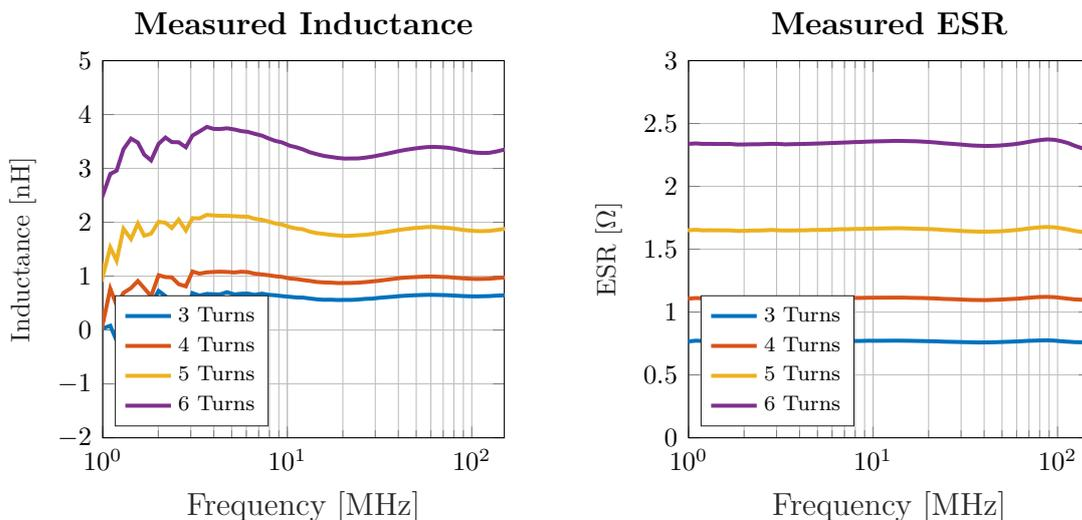
**Figure 5.3:** The extracted inductance and ESR from  $S$ -parameter measurements for four different S-inductors with a varying number of turns.
