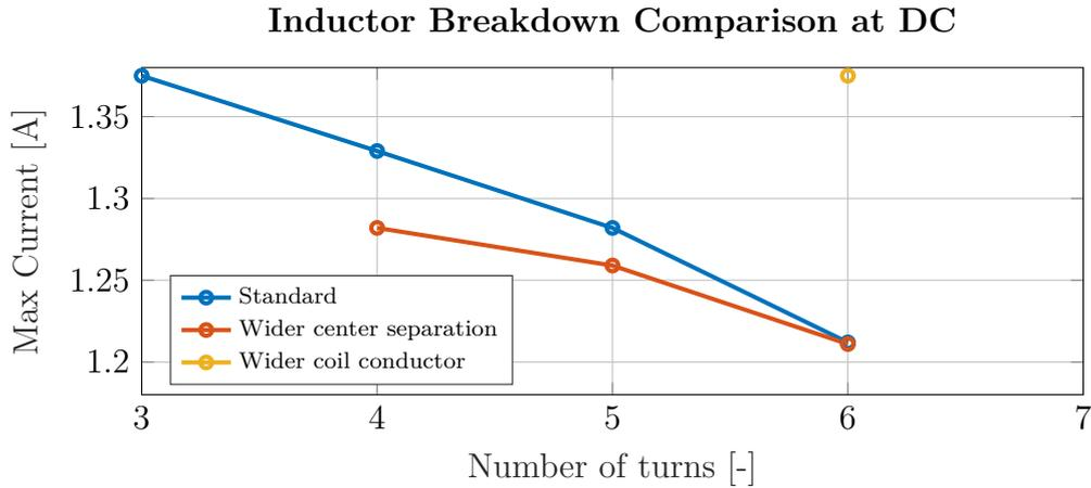
**Figure 5.11:** Measured breakdown current for the 9 different existing S-inductors.
