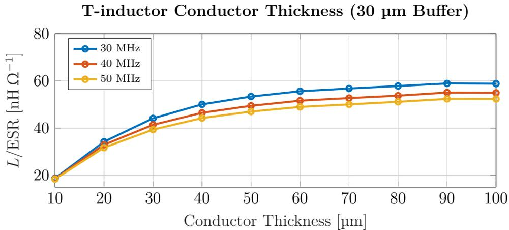
**Figure 5.10:** With a buffer thickness of 30  $\mu\text{m}$  the same decrease in  $L/\text{ESR}$  with decreasing conductor thickness is observed.
