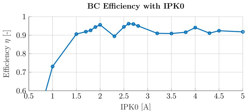
**Figure 4.3:** Efficiency of the BC with different IPK0 for the Angelov transistor model.
