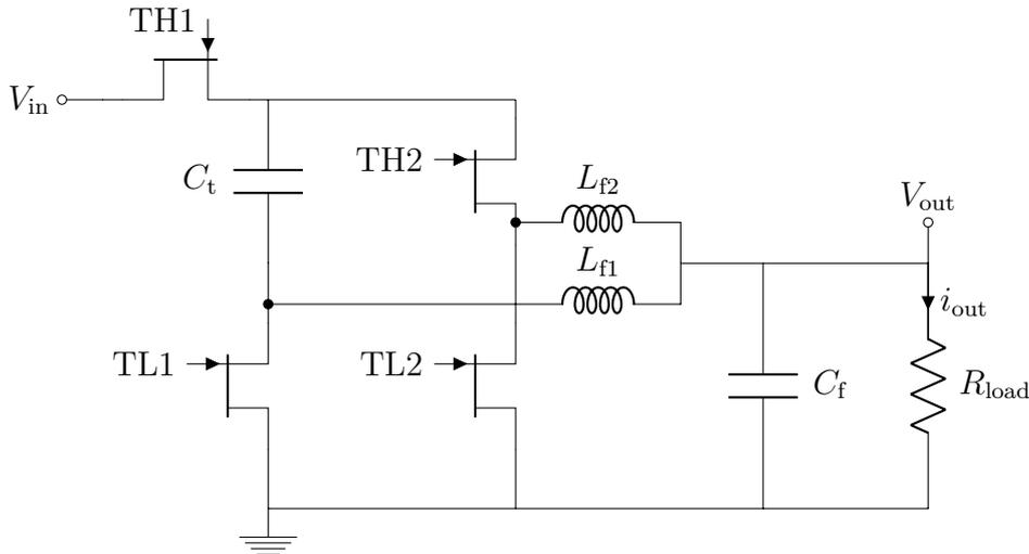
**Figure 3.10:** Schematic overview of the Modified Interleaved Buck Converter topology.
