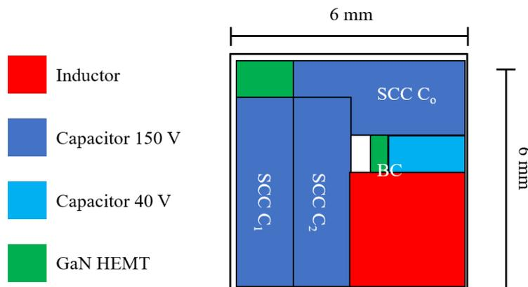
**Figure 6.13:** The circuit area required by each component for implementing a SCC and BC combination converter with T-inductors.
