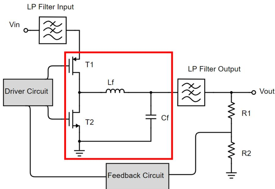
**Figure 1.1:** The DC-to-DC power stage of a switched mode Buck converter highlighted in red. Together with the feedback circuitry, the transistor driver stage, input and additional output filtering the power stage converts a high DC voltage  $V_{in}$  to a low lower DC voltage  $V_{out}$ . Not shown is a possible galvanic isolation stage that could be added as a pre- or post-stage.
