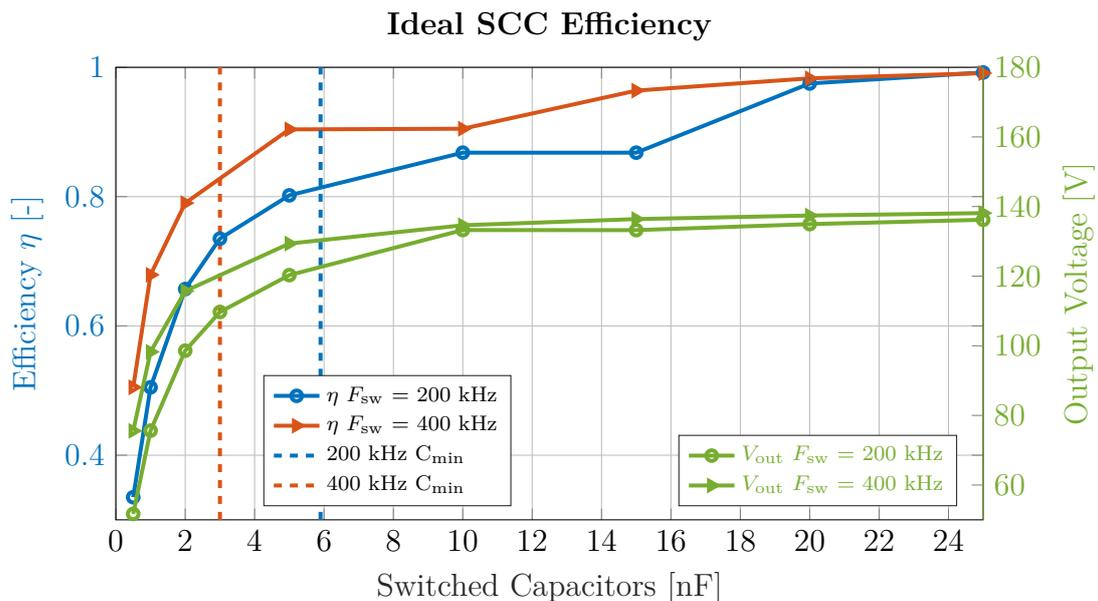
**Figure 4.16:** The efficiency and output voltage of an ideal SCC at 200 kHz and 400 kHz. Also indicated are the theoretical minimum capacitance values needed for 25 W output power from Figure 3.3.
