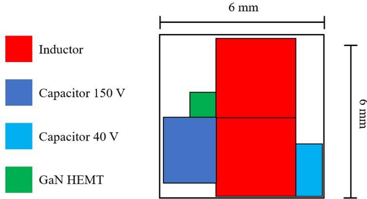
**Figure 6.9:** The size of each component type for an MIBC realized with T-inductors with  $30\ \mu\text{m}$  conductor thickness operating at 60 MHz.
