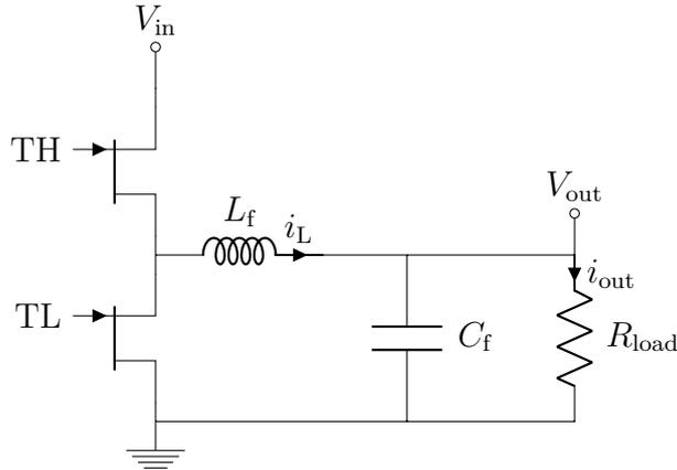
**Figure 3.5:** Schematic view of a synchronous Buck converter. Different control signals are fed to the gates of transistors TH and TL to make them act like opposing switches.
