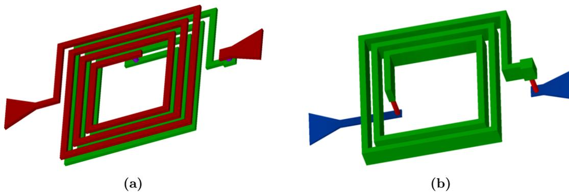
**Figure 5.2:** An example multi-layer inductor with ports in M3 (brown) and vias connecting to M2 (a). A thick inductor with ports in M1 (blue) and spiral windings in M2 (b).
