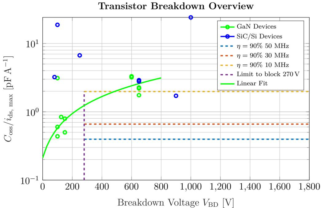
**Figure 6.1:** Performance metrics for devices in GaN, Si and SiC together with a linear fit between the two groups of GaN devices and efficiency boundaries for a conventional BC with regards to  $C_{\text{oss}}$  loss only. More details of the devices in Appendix A.
