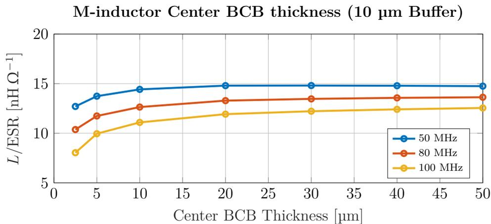
**Figure 5.6:** The thickness of the BCB layer that separates the two conductor layers in the M-inductors and the resulting  $L/\text{ESR}$ -ratio. (10  $\mu\text{m}$  buffer thickness)
