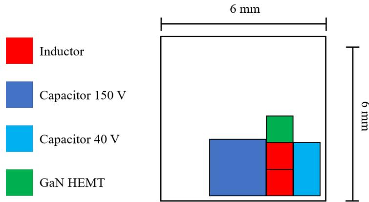
**Figure 6.7:** An approximate plot of the area requirement for each component type for realizing an MIBC in the M-technology.
