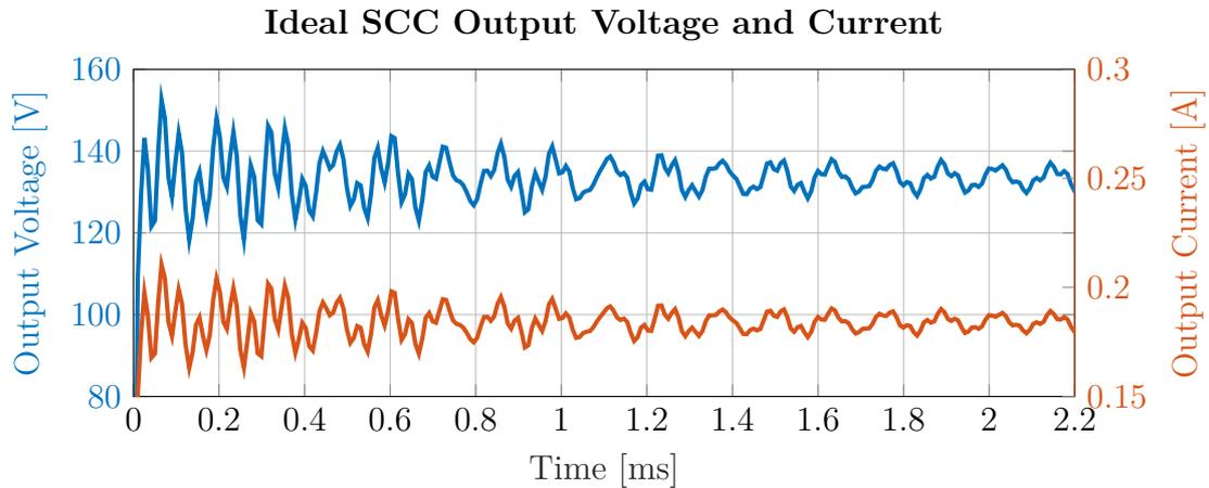
**Figure 4.15:** The output voltage and current as the SCC reaches steady state at  $f_{sw} = 400$  kHz with  $C_1 = C_2 = 15$  nF and  $C_o = 20$  nF.
