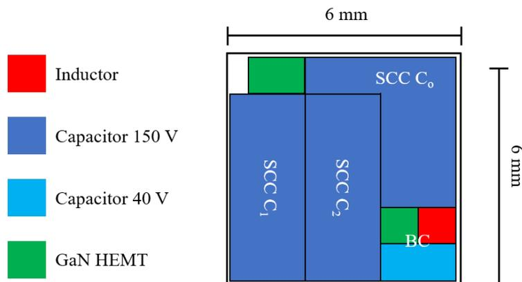
**Figure 6.11:** A schematic view of the approximate space requirements for the different components of the BC and SCC combination. Realized in the M-technology.
