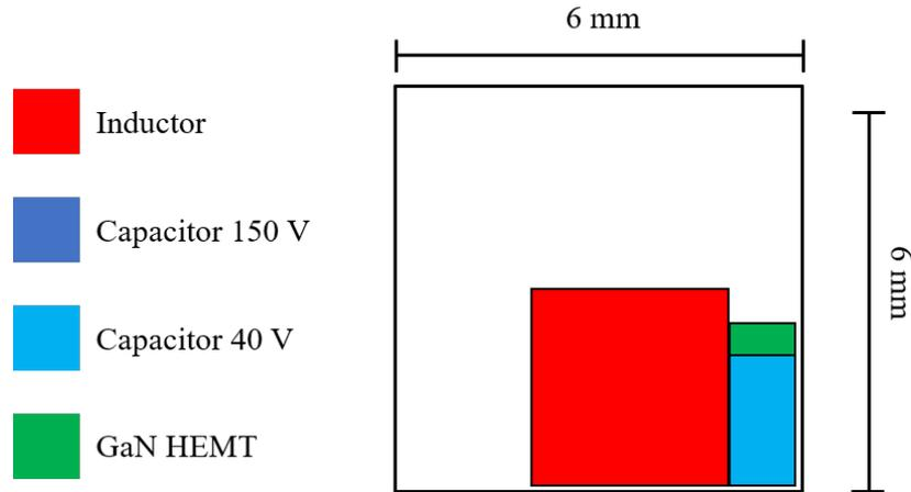
**Figure 6.5:** The approximate component area for a conventional BC realized with T-inductors with 30  $\mu\text{m}$  conductor thickness.
