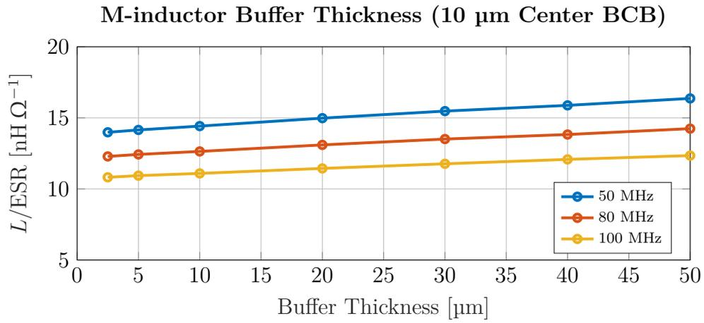
**Figure 5.7:** Performance ( $L/ESR$ ) for the M-inductors with buffer BCB thickness.
