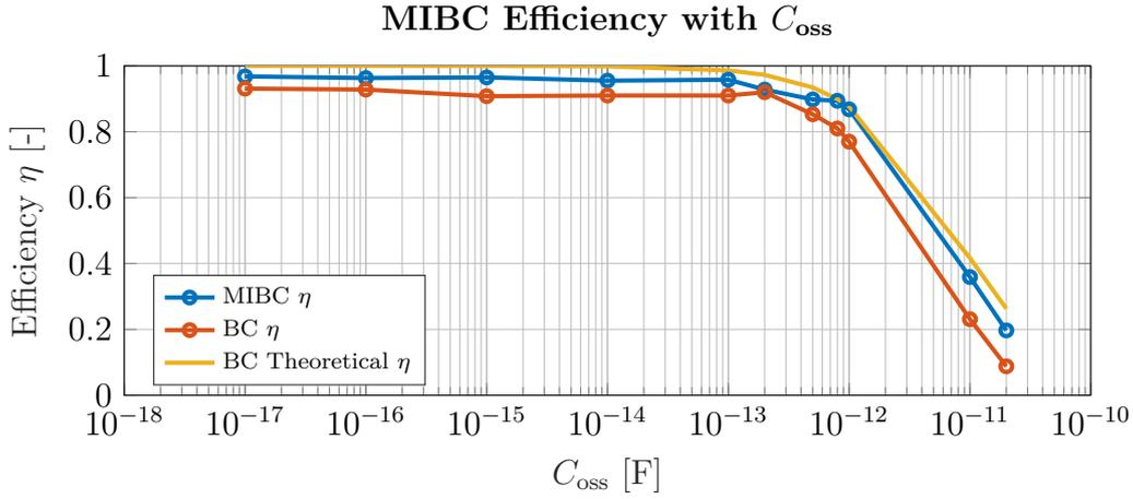
**Figure 4.11:** Simulated efficiency  $\eta$  for the MIBC at 50 MHz with increasing output capacitance  $C_{oss}$ , compared to the BC and the theoretical curve.
