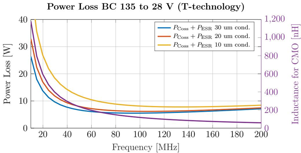
**Figure 6.12:** The power loss for a 135 to 28 V BC realized in T-technology with different conductor thicknesses.
