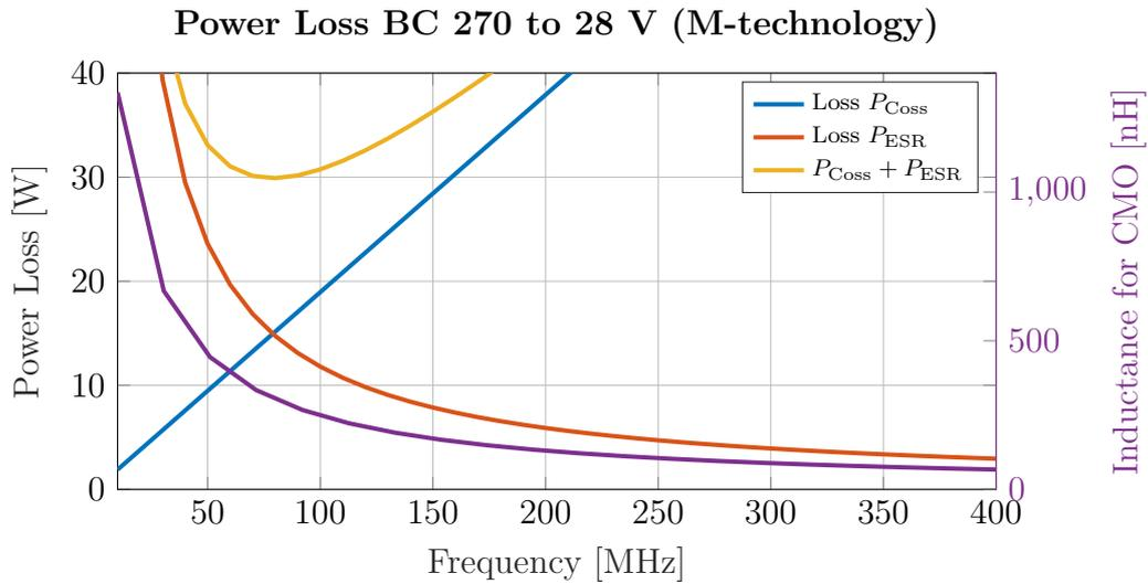
**Figure 6.2:** The power loss from inductor ESR and parasitic device capacitance as a function of frequency for a BC realized in the M-technology, at an output power of 26.3 W.
