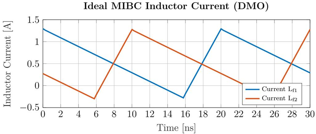
**Figure 4.8:** Flywheel inductor current through each branch of the MIBC for  $L_{f1} = L_{f2} = 300 \text{ nH}$  at steady state ( $t + 10 \mu\text{s}$ ). The converter is in FCMO.
