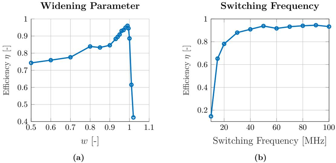
**Figure 4.6:** BC efficiency for different  $w$  of the control signal to TL (a) and the simulated efficiency of the ideal Buck Converter operating at different switching frequencies (b).
