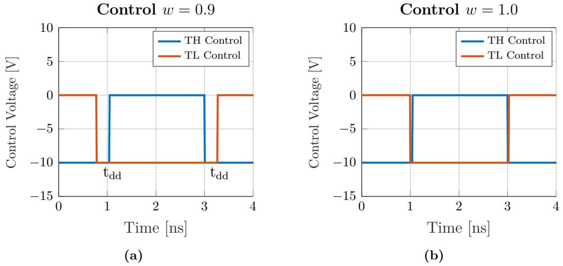
**Figure 3.11:** The control signals for the high and low side transistor in a BC with widening parameter  $w = 0.9$  makes the OFF state for the low side switch longer, introducing a dead time  $t_{\text{dd}}$  when both TH and TL are OFF (a). With no dead time,  $w = 0$ , there is a risk for conduction through both devices (b).
