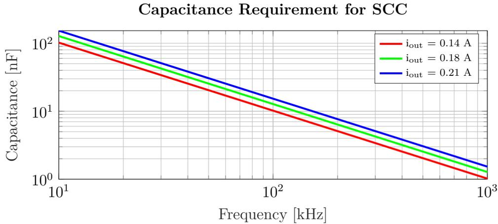
**Figure 3.3:** Required transfer capacitance values as a function of switching frequency for currents representing an output power of approximately 20 W, 25 W and 30 W respectively. Here  $V_{in} = 270$  V.
