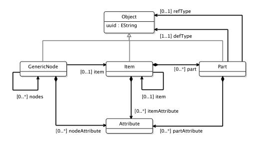
Figure 3.1: SystemWeaver meta-model of the conceptual architecture Source: SystemWeaver help documentation
