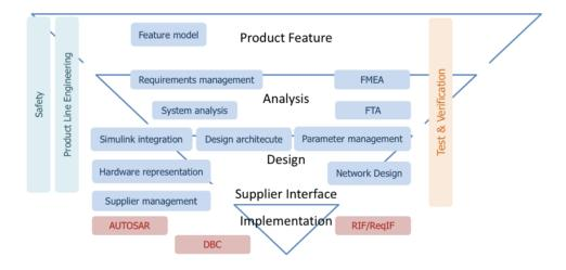
Figure 3.2: SystemWeaver integrated embedded system development process Source: SystemWeaver help documentation
