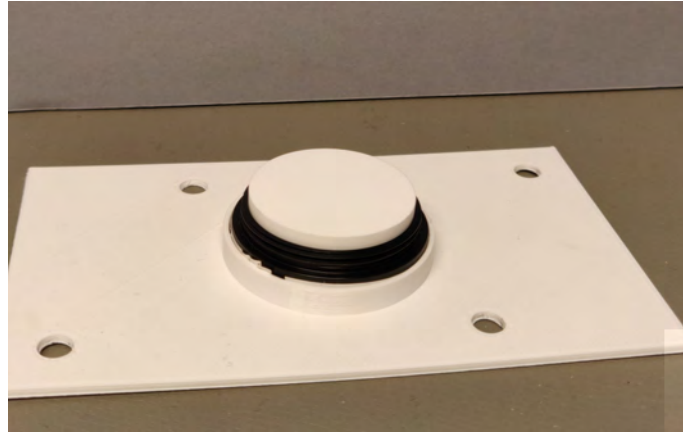
Figure 4.2: Spectralon material, calibrated to reflect more than 0.99 % of incoming light diffusely.
