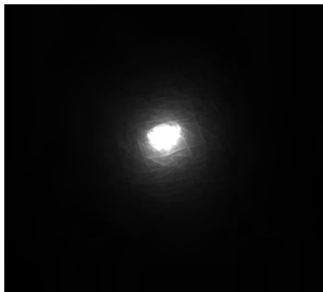
Figure 3.5: Human skin being illuminated by a focused point of near-infrared light.
