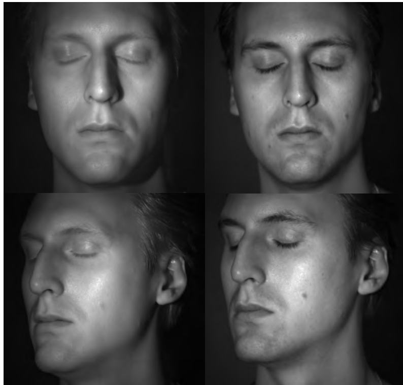
Figure 3.9: Left images are images of a face illuminated by near-infrared (940 nm) light while the right column of images are illuminated in visible light and then grayscaled by the camera.
