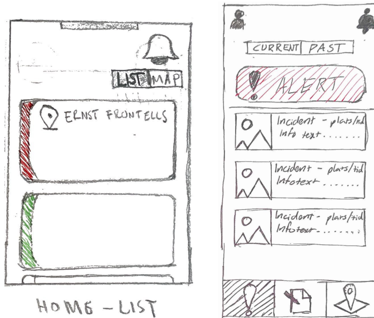
(a) A alerts feed that can be navigated to by selecting 'List' in the tab (alternative views pattern). (b) An alerts feed that can be navigated to through a dedicated 'alerts' icon.
